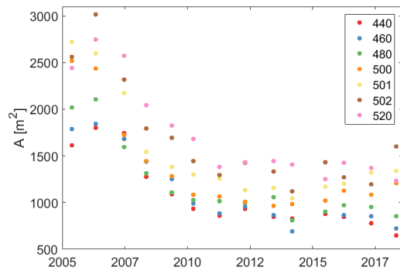
Figure 3.4: Development over time of current-carrying area of the Plaatgat below NAP -3 m till 2 000 m from the main beach pole ( RSP )
