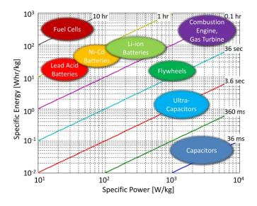
Figure B.1: Ragone plot of energy systems, the axes are logarithmic. Source: figure obtained from [32]
