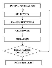
Figure 7.1: Loop of a genetic algorithm Source: figure obtained from [74]
