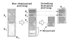
Figure 7.3: NSGA-II procedure Source: figure obtained from [23]
