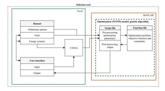
Figure 7.8: Flow chart of the selection tool (detailed version is given in Appendix F)
