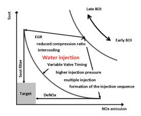
Figure 2.3: Trade-off for diesel engines between NO<sub>x</sub> and PM emissions. Source: figure obtained from [49]
