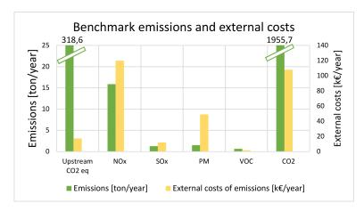
Figure 9.3: Benchmark (workboat) emissions and external costs, with the external costs shown on the secondary axis
