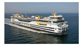
Figure 8.2: Double-ended road ferry TESO Texelstroom with two bridges. Source: figure obtained from [13].
