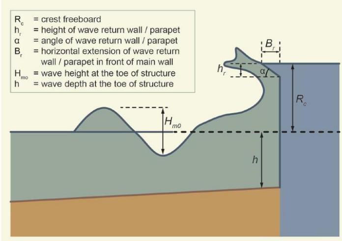
Figure 108 - Vertical wall with parapet (EurOtop, 2018)
