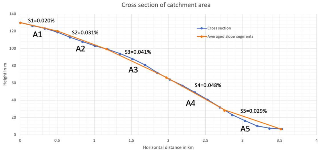
Figure 29 - Cross section of catchment area
