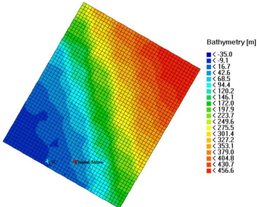
Figure 87 – XBeach Bathymetry grid and Observation point for significant wave height
