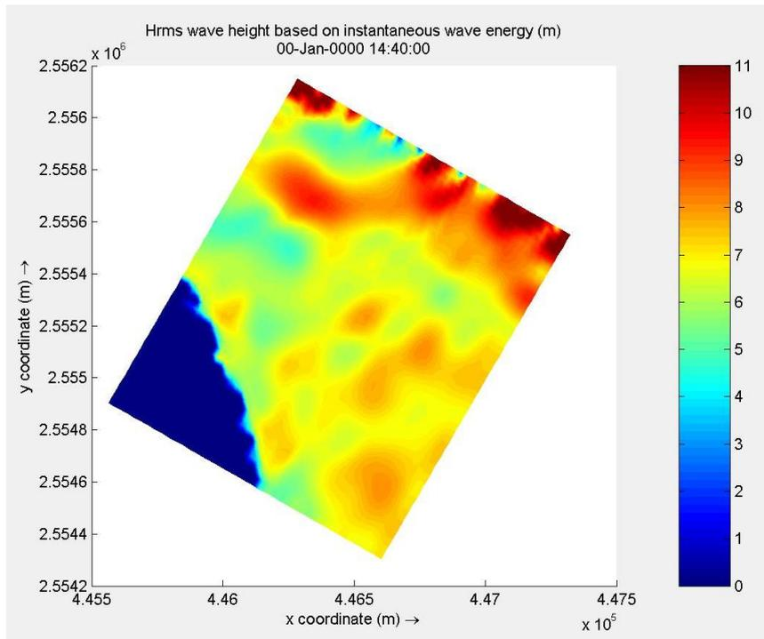
Figure 104 - Significant wave heights combination 2, XBeach
