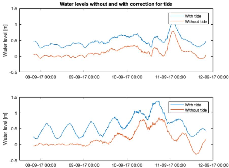
Figure 74 - Water levels with and without tide
