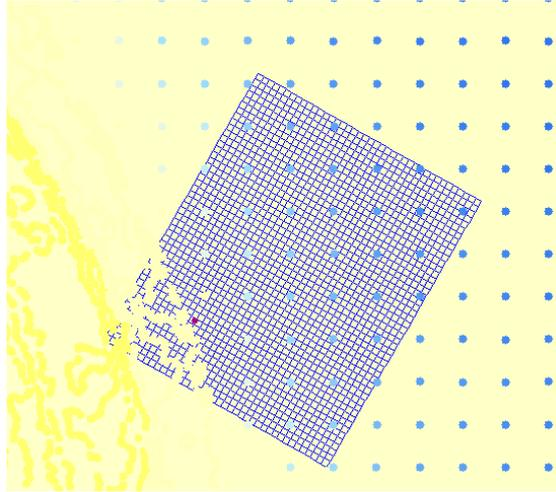
Figure 78 – XBeach grid with bathymetry and CTE indicated
