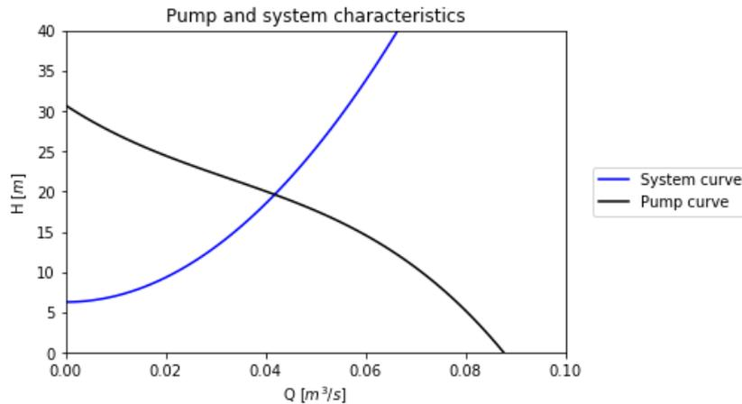
Figure 143 – Pump and system curves
