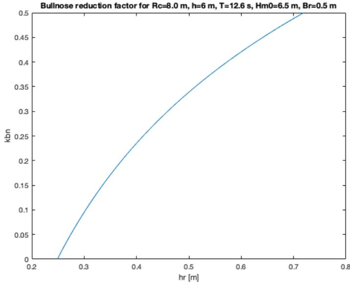
Figure 155 – Bullnose reduction factor versus the bullnose height for the parameters of the coastal defense at cross section A
