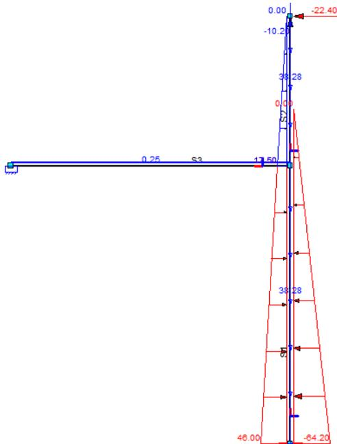
Figure 158 - Load case full stilling basin and full wave impact
