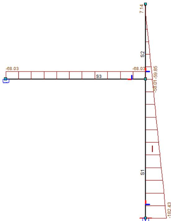
Figure 233 - Normal force, empty basin full wave impact
