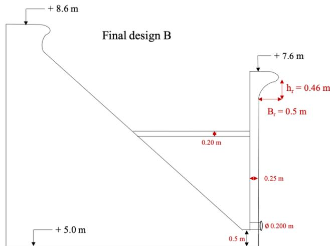
Figure 151 - Final design cross section B
