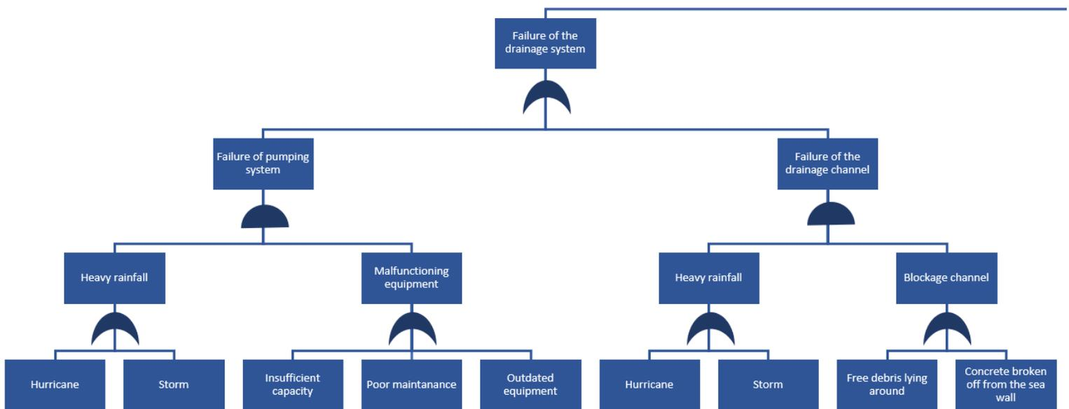
Figure 186 – Failure of the drainage system
