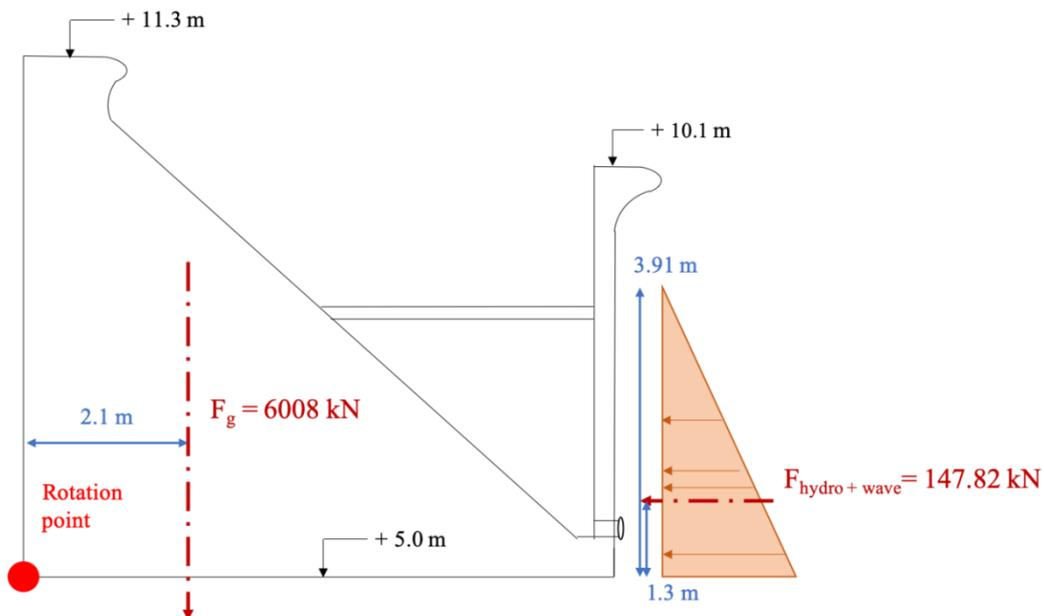
Figure 167 – Rotational stability of the new design
