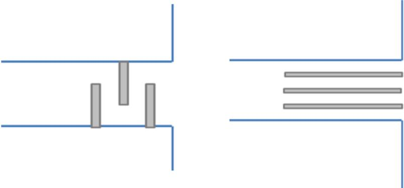
Figure 148 – Possible lay out of the wave attenuation channel
