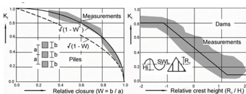
Figure 133 - Pile screen wave reduction
