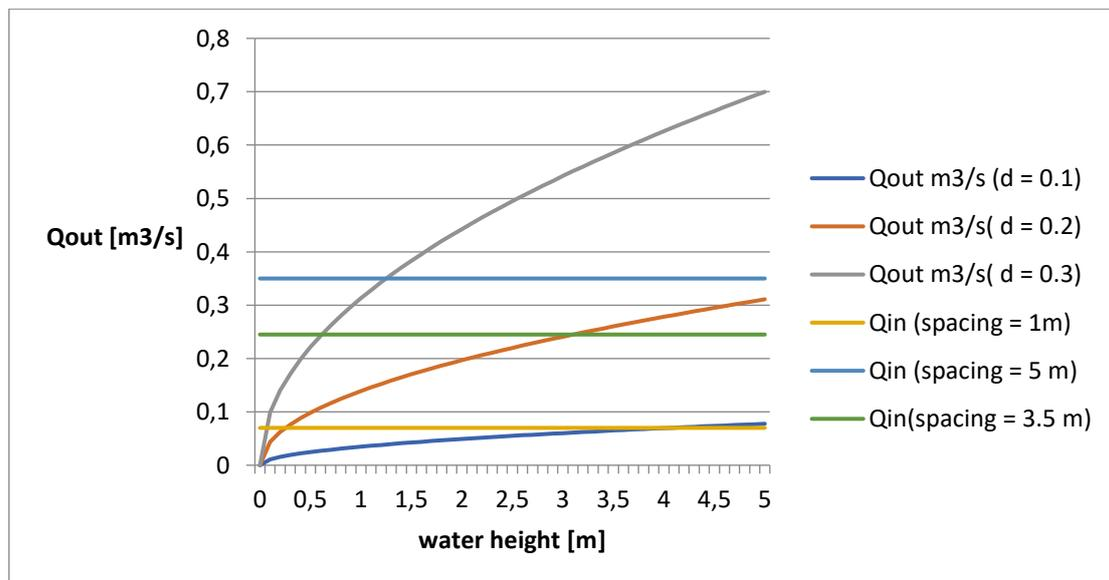
Figure 173 - Discharge vs water height
