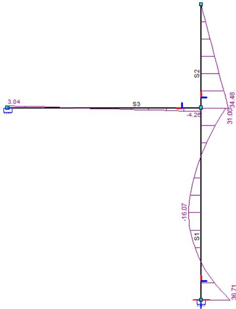
Figure 161 - Moment distribution empty tank, full wave impact
