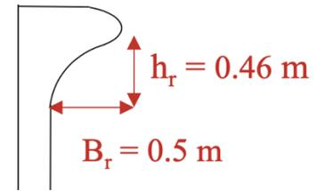
Figure 156 – Bullnose geometry
