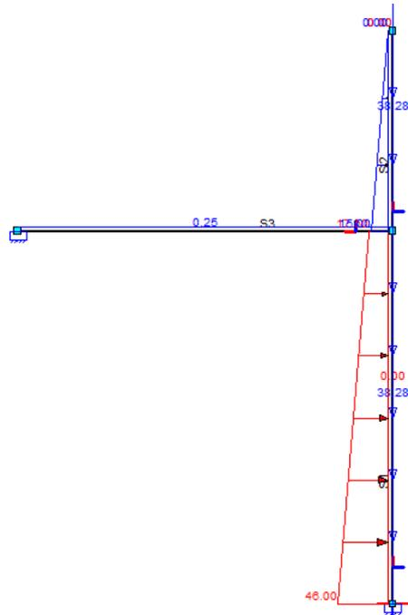
Figure 159 - Load case full stilling basin no wave impact
