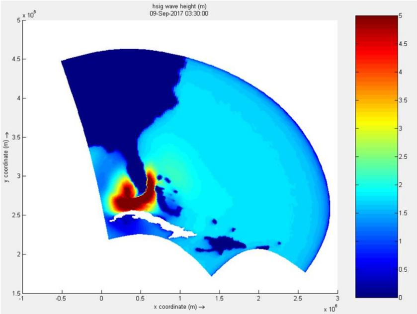
Figure 103 - Combination 2, distribution significant wave heights over the whole area
