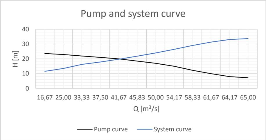
Figure 145 - Pump and system curve
