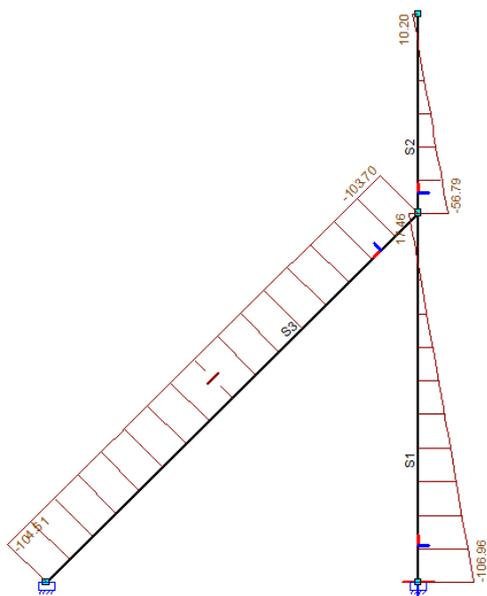
Figure 245 - Normal force diagram wall inlet channel, only wave impact
