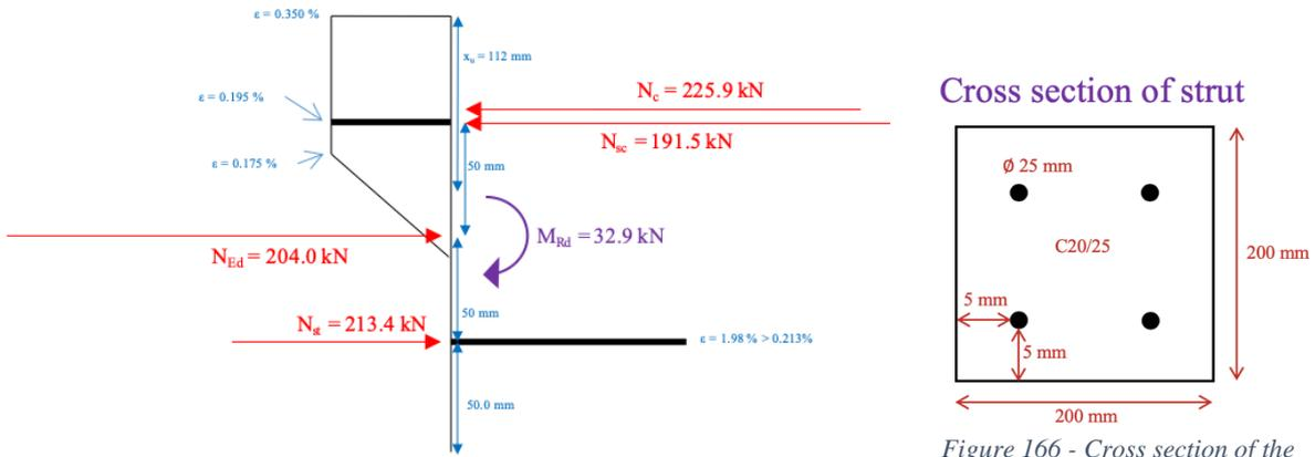
Figure 165 – Cross section with its forces of the strut
