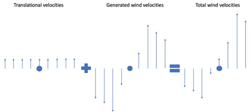
Figure 63 - Schematization of asymmetrical wind field
