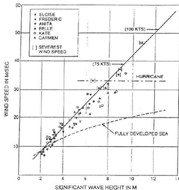
Figure 16 - Significant wave height vs wind speed moderate seas (Ochi, 1993).
