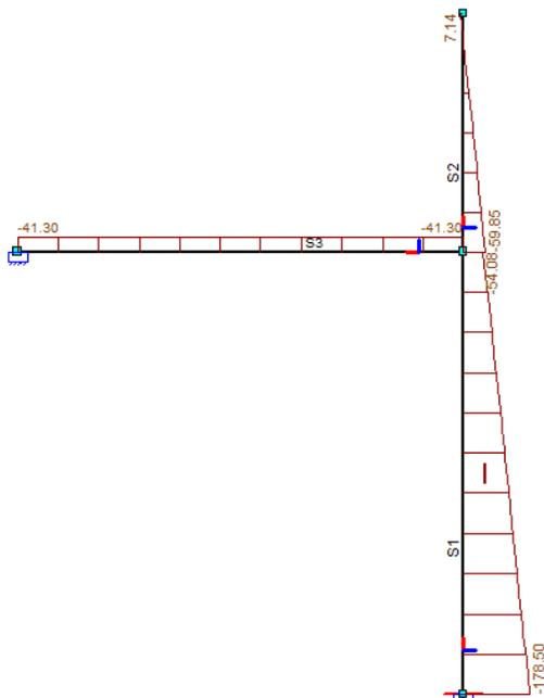
Figure 236 - Normal force diagram  $h = 4$  m
