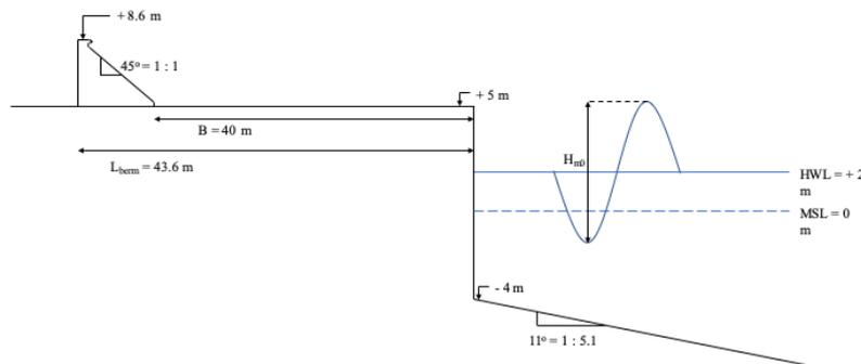
Figure 116 - Schematization section B
