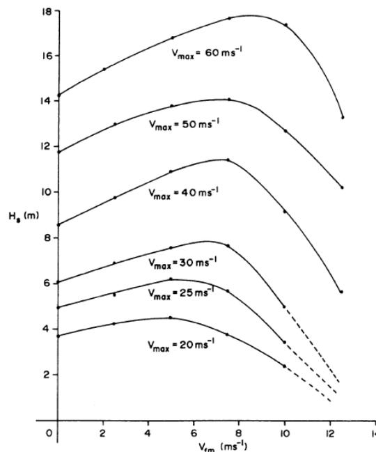
Figure 18 - Significant wave height vs  $V_{fm}$  for different  $V_{max}$  (Young, 1988)
