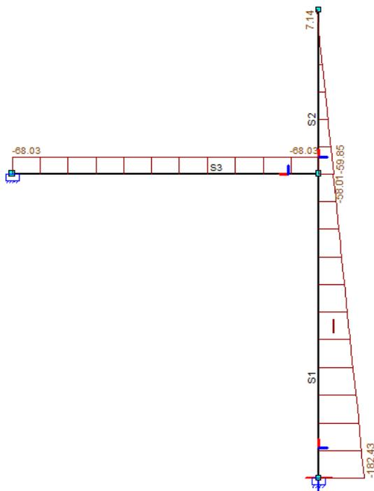
Figure 163 - Normal force, empty basin full wave impact
