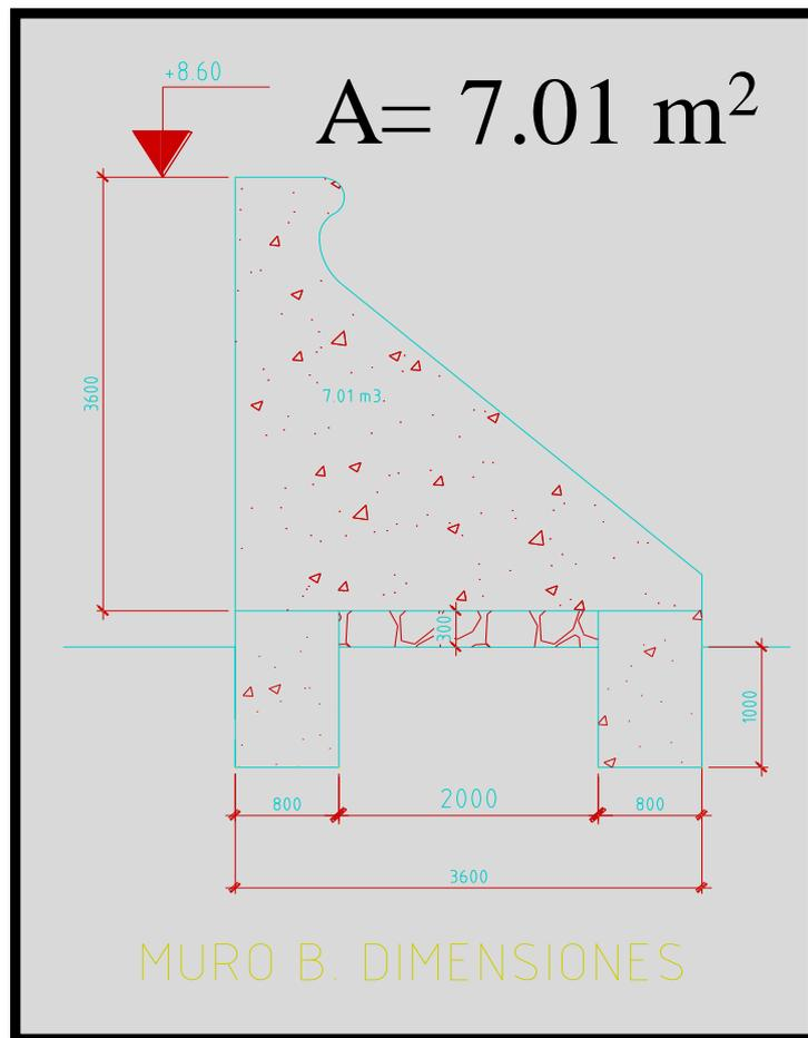
Figure 184 – Technical drawing of the current defense wall part B
