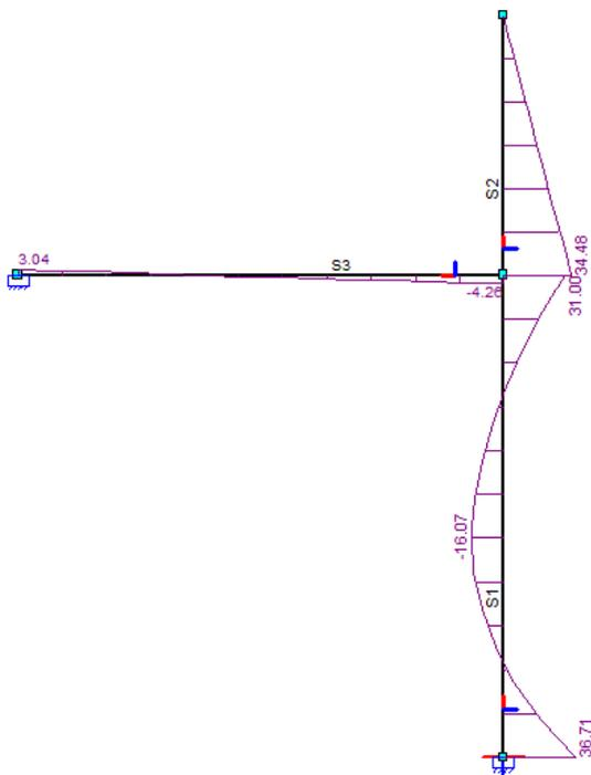
Figure 230 - Moment distribution empty tank, full wave impact
