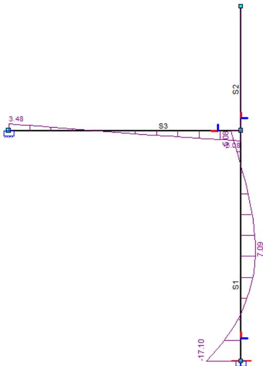
Figure 240 - Moment distribution,  $h = 3$  m, no wave
