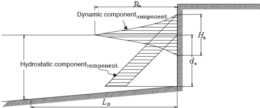
Figure 153 - Method Minikin broken waves pressure (TU Delft, 2019)
