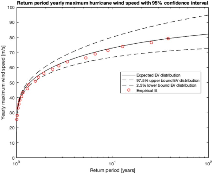
Figure 35 – GEV fit wind speeds
