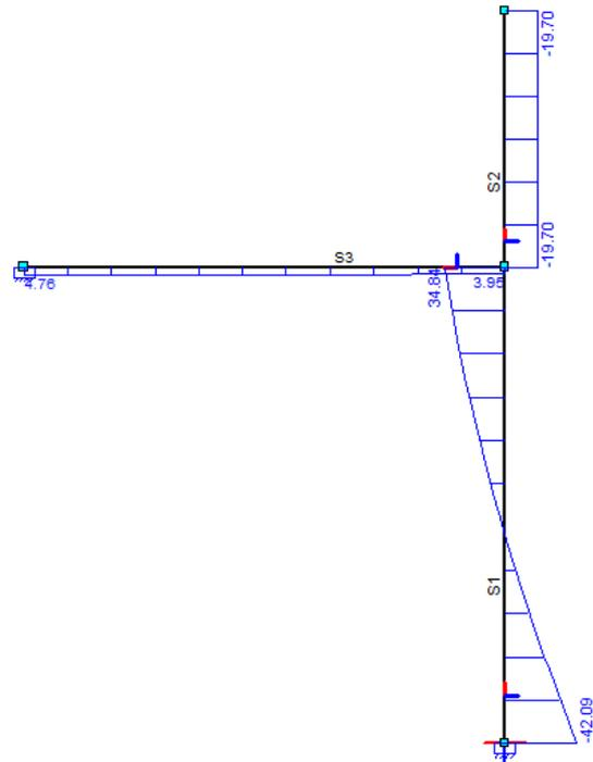
Figure 238 - Shear force diagram,  $h = 3$  m, wave impact
