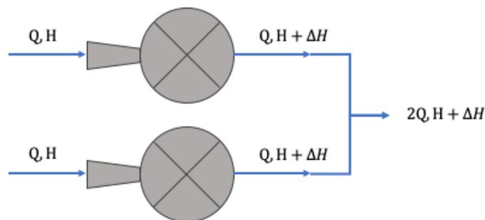
Figure 141 – Pumps in parallel
