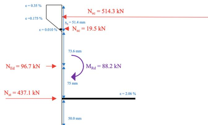
Figure 168 – Moment resistance capacity of cross section at the governing normal force
