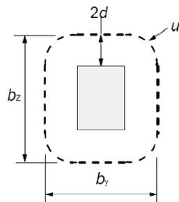
Figure 172 - Sketch basic control perimeter
