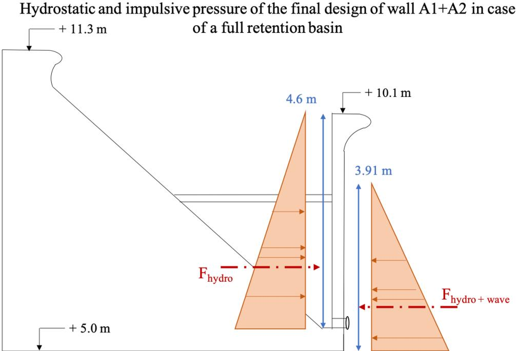
Figure 154 - Schematization hydrostatic pressures
