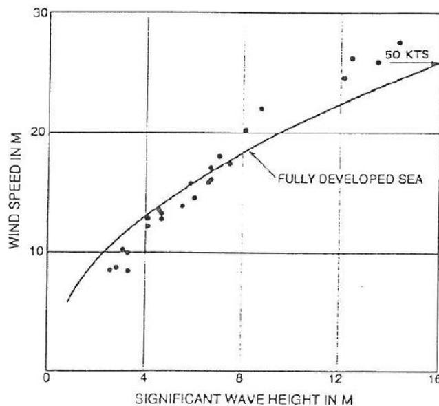
Figure 17 - Significant wave height vs wind speed hurricane Gloria (Ochi, 1993)
