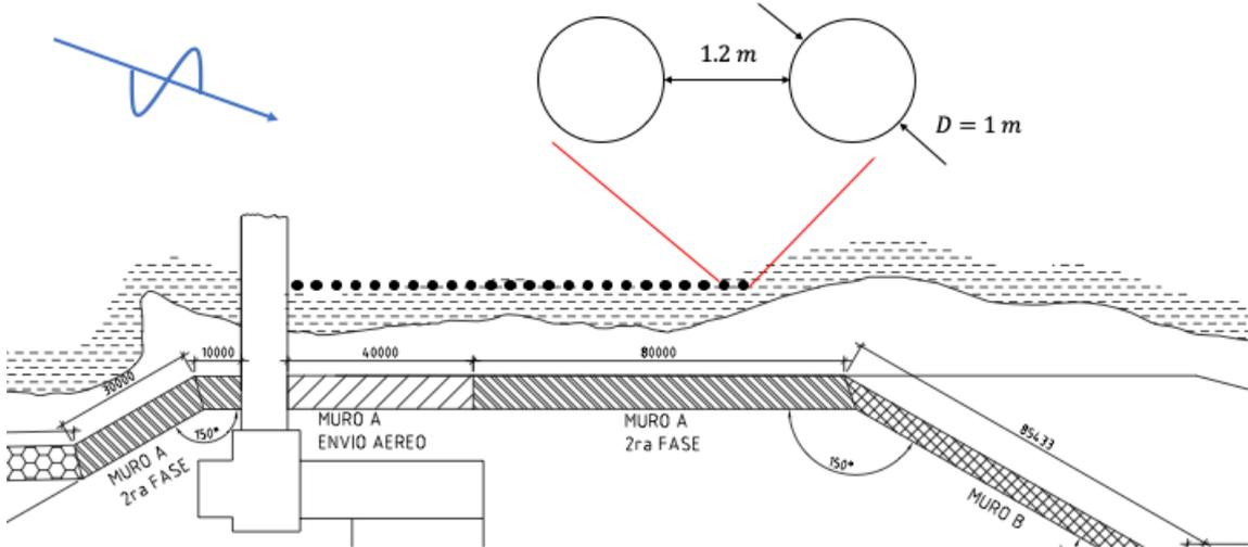
Figure 134 - Section A-1 pilescreen lay out
