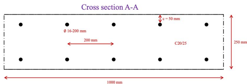
Figure 164 - Cross section of a unit width of 1000 mm wide of the coastal protection
