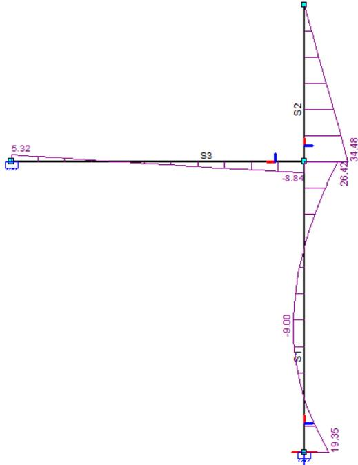
Figure 237 - Moment distribution,  $h = 3$  m, wave impact
