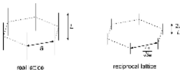
Figure 3.16. Transformation of a real hexagonal lattice of finite rods into its reciprocal lattice.
