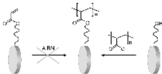
Figure 1. Schematic presentation of the polymer synthesis: the approach of polymerization of the acrylic functional mesogen under free-radical conditions or a polymer analogous reaction with poly(acryloyl chloride).
