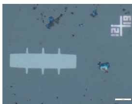
Figure 3.15: Freestanding NNO Hall bar stamped on sapphire after removal of the additional protective PMMA layer via acetone. A pre-patterned platinum alignment marker can be seen in the upper right. Polymer residues remain which proved resistant to O 2 plasma treatment as well as xylene wet etching.
