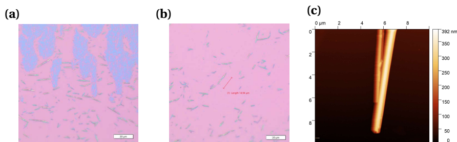
Figure 3.19: (a) 50x optical image of LAO/BTO membrane stamped onto a Si substrate. The cylindrical objects are LAO/BTO nanoscrolls that formed after stamping. (b) Optical image of nanoscrolls, with length scale provided. (c) AFM image of a LAO/BTO nanoscroll
