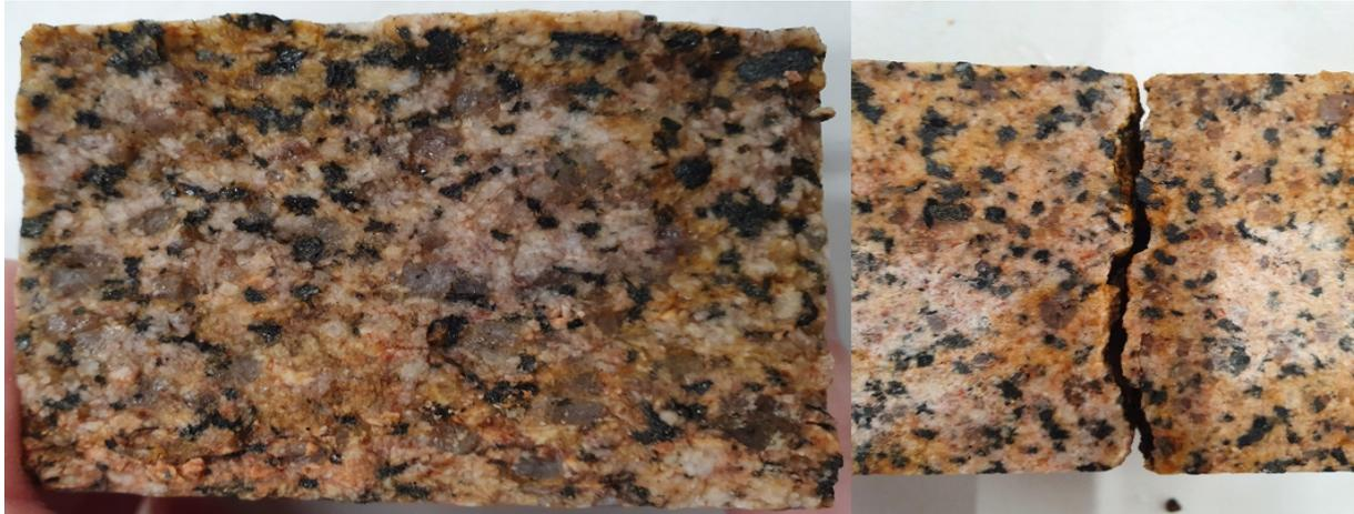
Figure 3.16: Rough, tensile-split sample as seen from the top (left) and side (right). From these pictures, it can be seen that there is a difference in color between the outside and inside of the material. This is likely caused by weathering of the rock.
