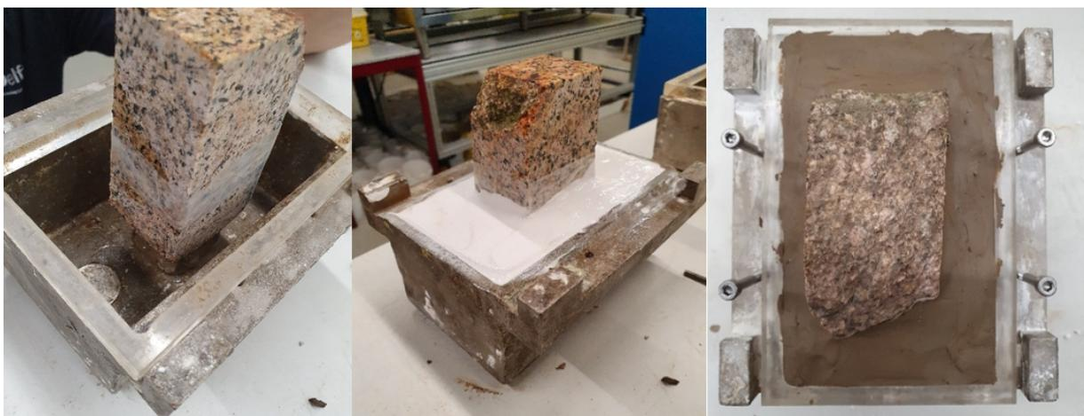
Figure 3.17: Sample preparation with clay and gypsum.
