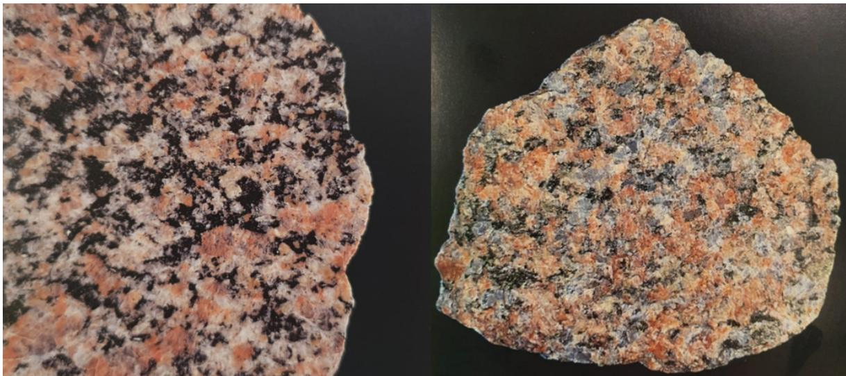
Figure 3.2: Grey Väjö granite (left) and red Väjö granite (right). Adopted and modified from (Zandstra, 1999).
