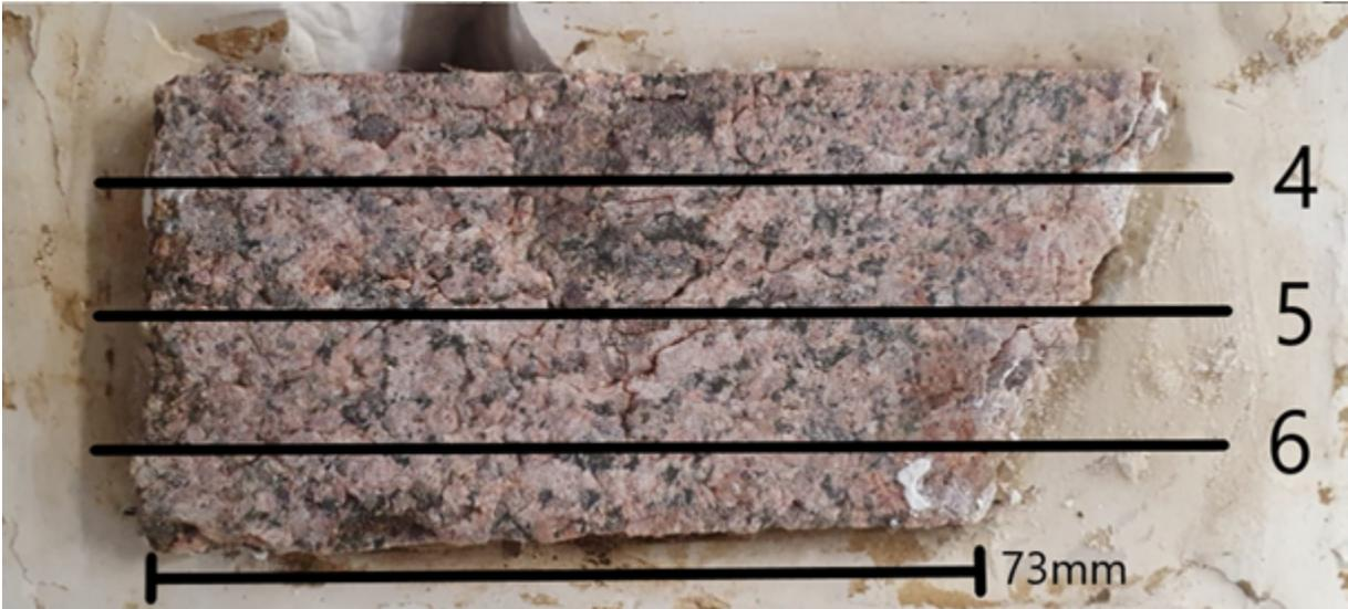
Figure L.7: Overview of the roughness profiles on the flat top sample.
