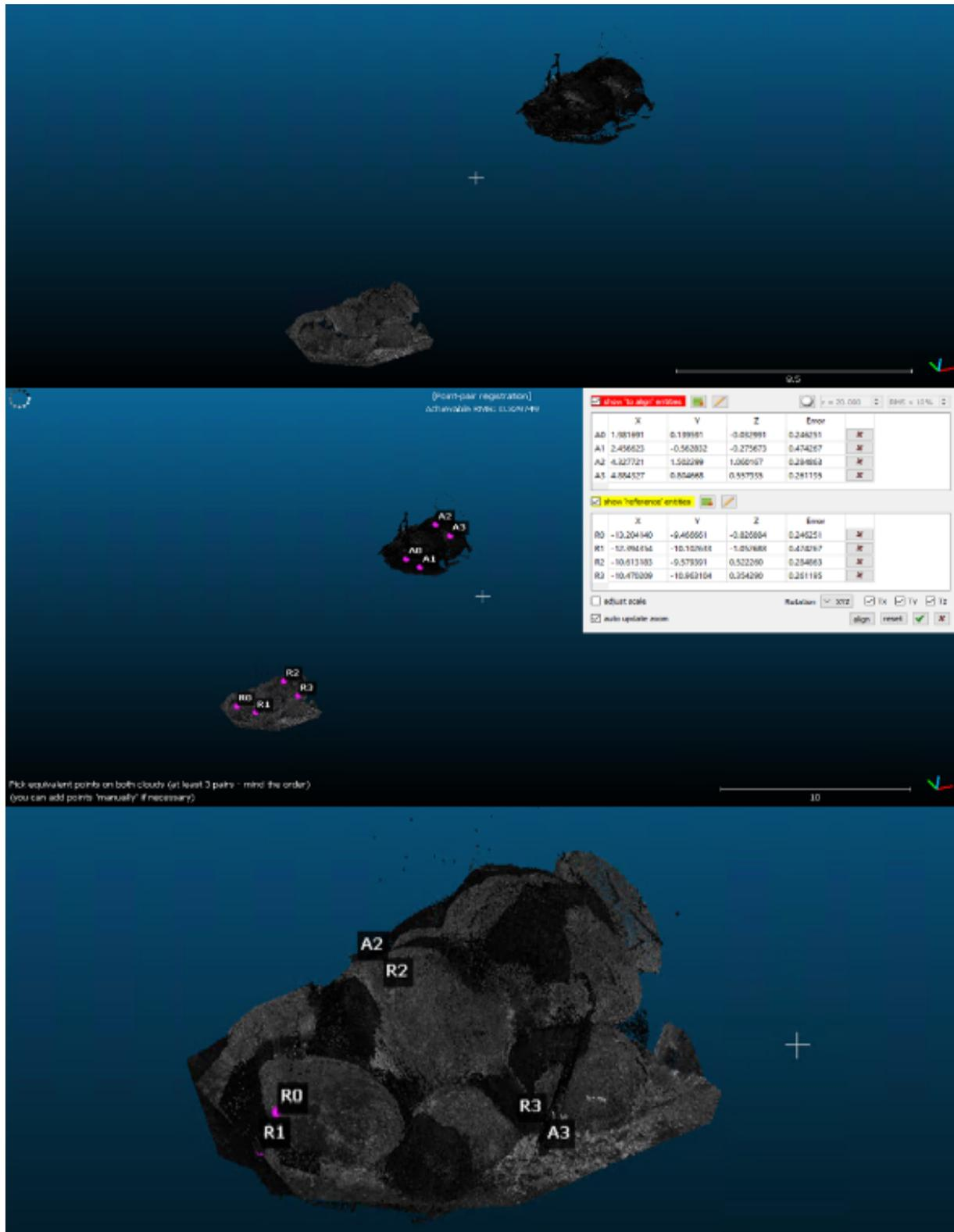
Figure B.2: Illustration of point cloud modelling Step 2.2: Align BLK data to TLS data set. The scale of the figure is indicated in meters.
