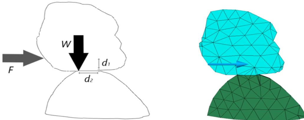
Figure 4.5: Dolmen D14 in 2D at the Northern contact point between Rock 3 and Rock 2: schematic for analytical calculations (left) and numerical model (right).
