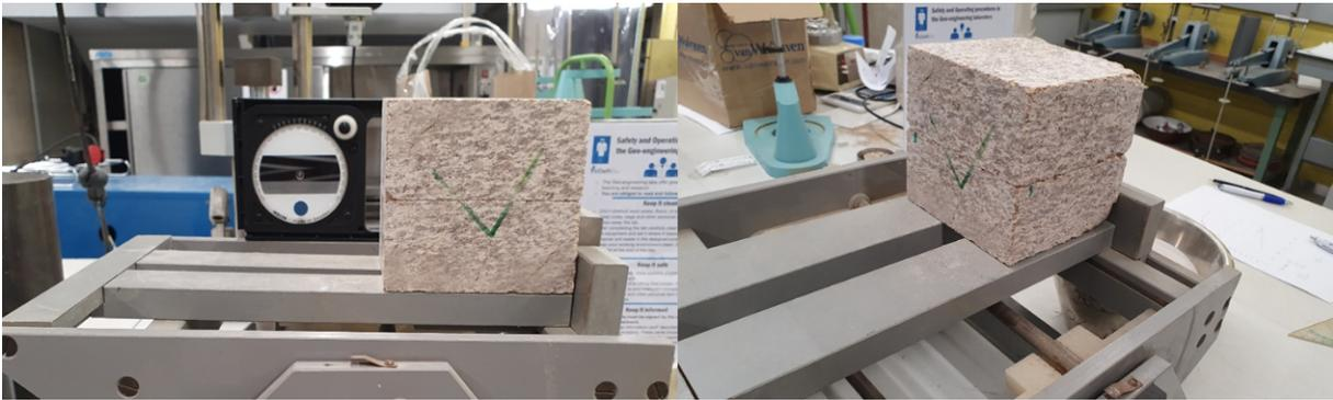
Figure K.1: Tilt test performed on the flat, sand-blasted granite sample in direction 1 (left) and direction 2 (right).
