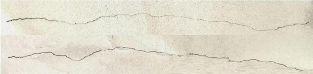
Figure I.7: Roughness profile Rock 4. Profile 1 (top) and profile 2 (bottom).
