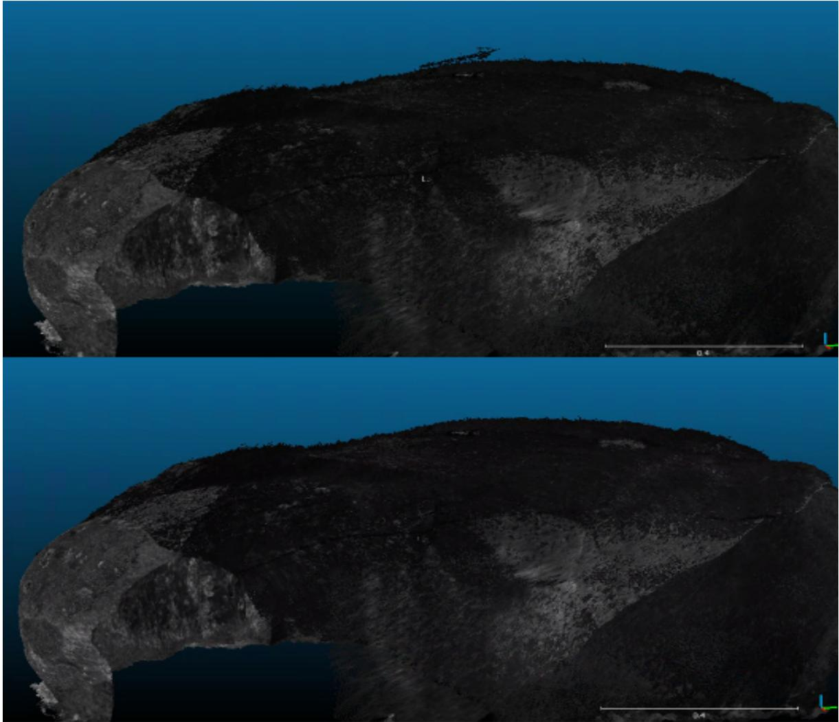
Figure B.7: Illustration of point cloud modelling Step 2.7: Clean the data set. The scale of the figure is indicated in meters.
