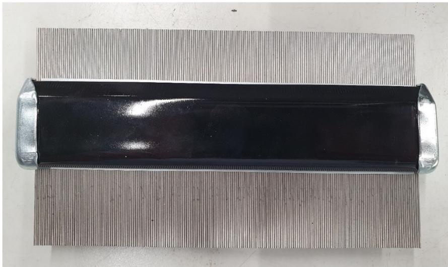
Figure 3.11: The Barton's comb that was used to obtain the roughness profiles. The diameter of one pin is approximately 0.8mm and the distance between pins is approximately 1mm.
