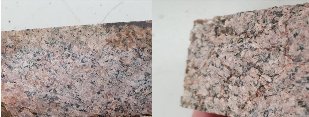
Figure 3.14: Sawed surface of the rock sample before (left) and after (right) sandblasting. It can be observed that there are more small cracks along grain boundaries in the surface after sand-blasting.
