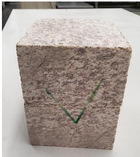
Figure 3.12: Tilt test sample.
