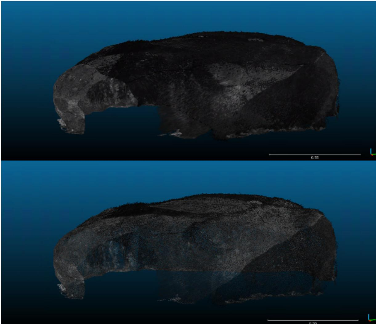
Figure B.8: Illustration of point cloud modelling Step 2.8: Subsample. The scale of the figure is indicated in meters.
