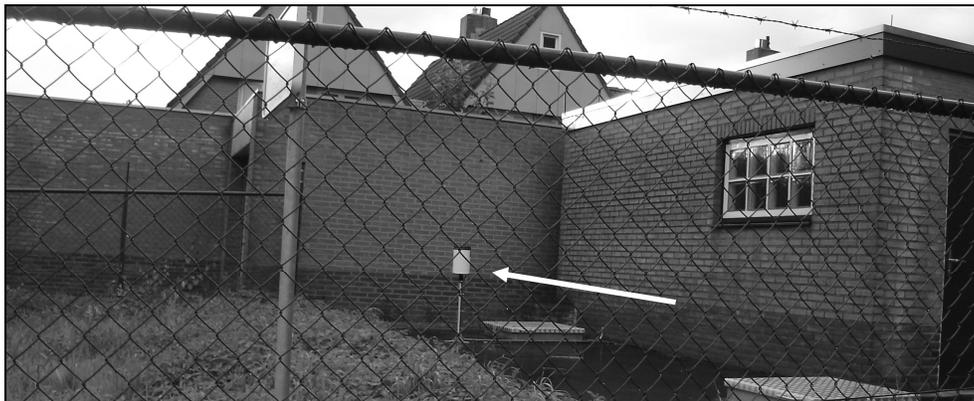
Figure 3-2: WDD rain gauge in Heeze placed directly next to the pumping station building
