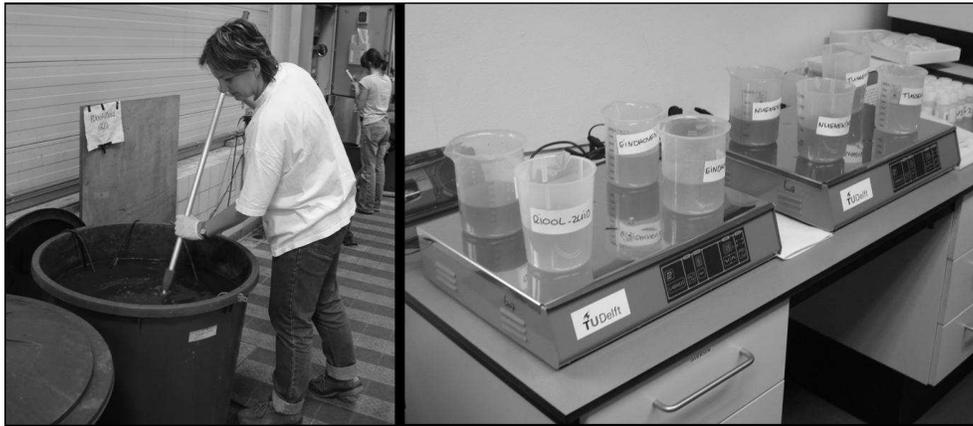
**Figure 5-7:** (left picture) taking a grab sample from a measurement vessel holding a UV/VIS sensor; (right picture) samples from inflows Riool-Zuid, Eindhoven Stad and Nuenen/Son at the magnetic stirrer ready for laboratory analysis (at the far end, samples from a fourth location ‘tussengemaal’, results of which are not presented in this thesis)
