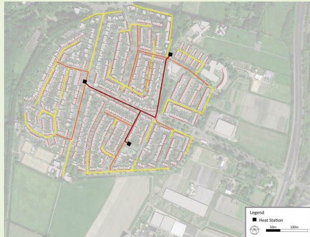
Figure 5.34: Map of alternative heat network layout with connections along the drains and eaves (Own ill.)
