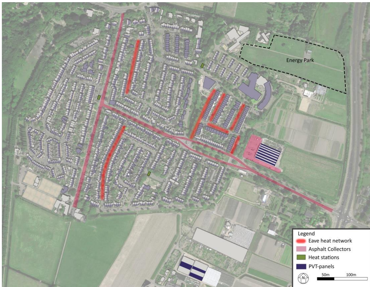
Figure 6.1: Map with interventions highlighted of the minimal and (plus the energy park) optimal scenario
