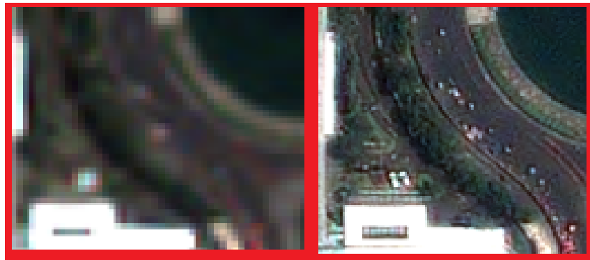
Figure 13: Zoomed-in image taken from Figure 12. Multispectral image (left) vs. pan-sharpened image (right).
