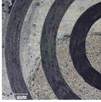
(b) The wear track of different radius, 3.016, 5.603, and 8.038 mm.
