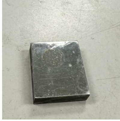
(b) HVAF Hastelloy C276 with 2-layer \text{SiO}_2/\text{ZrO}_2 sol-gel sealing layer
