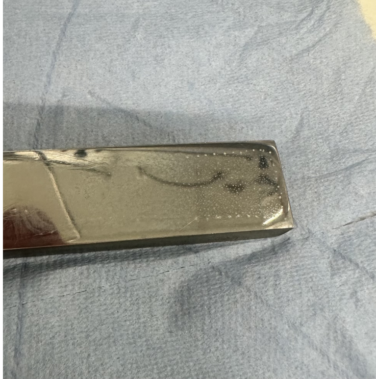
Figure 15: The white particles which can be seen on Hastelloy C22.
