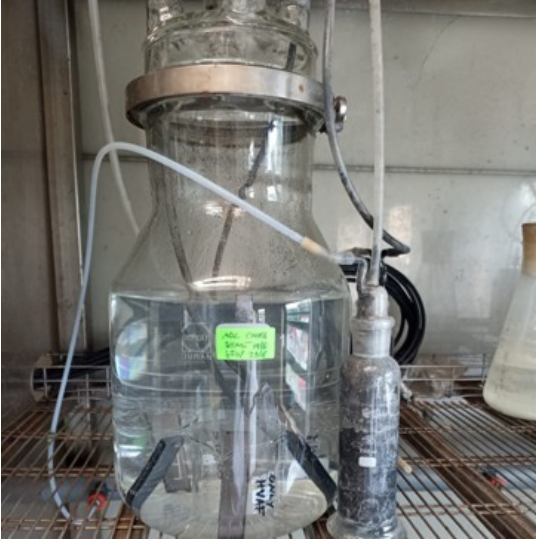
(a) Equipment setup for the immersion test, and all samples are inside the test container.
