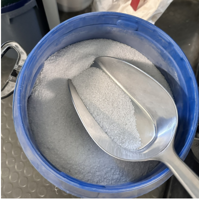
(a) Corundum F-20 powder for grit blasting.
