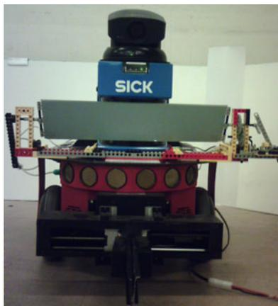
Figure 2.1: This picture show the 2D laser scanner and the 3D rotation mechanism on the robot [62].
