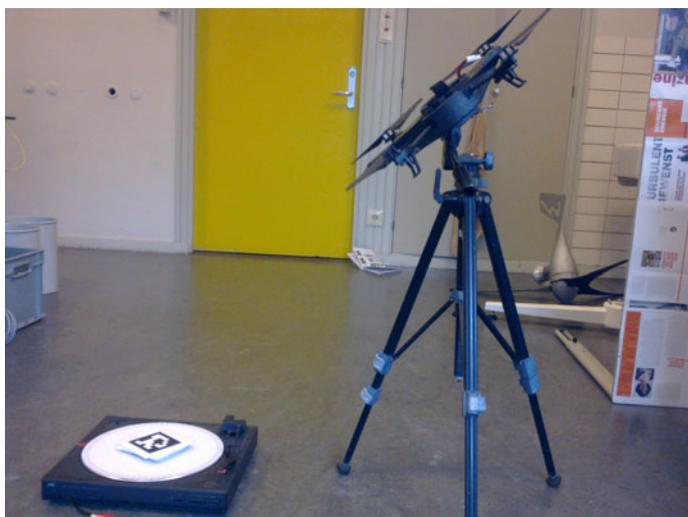
Figure 5.2: This picture shows the test setup used in experiment 5.1. The marker is rotated at low speed while the quadrotor is moved.
