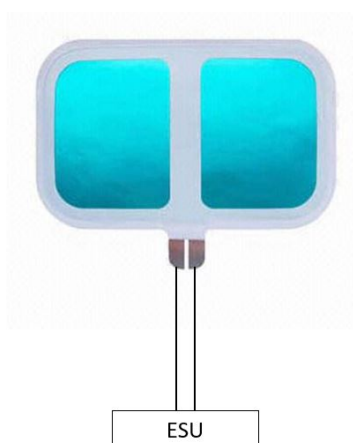
Figure E.1: Schematic drawing of the return electrode, based on [19]
