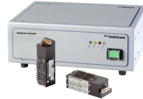
Figure 2.5: Pressure scanning system DTC Initium in LTT. Source: https://www.te.com/en/product-CAT-SCS0010.html .
