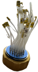
Figure 2.4: Pressure tubes connected to a connector that attaches to the DTC Initium.
