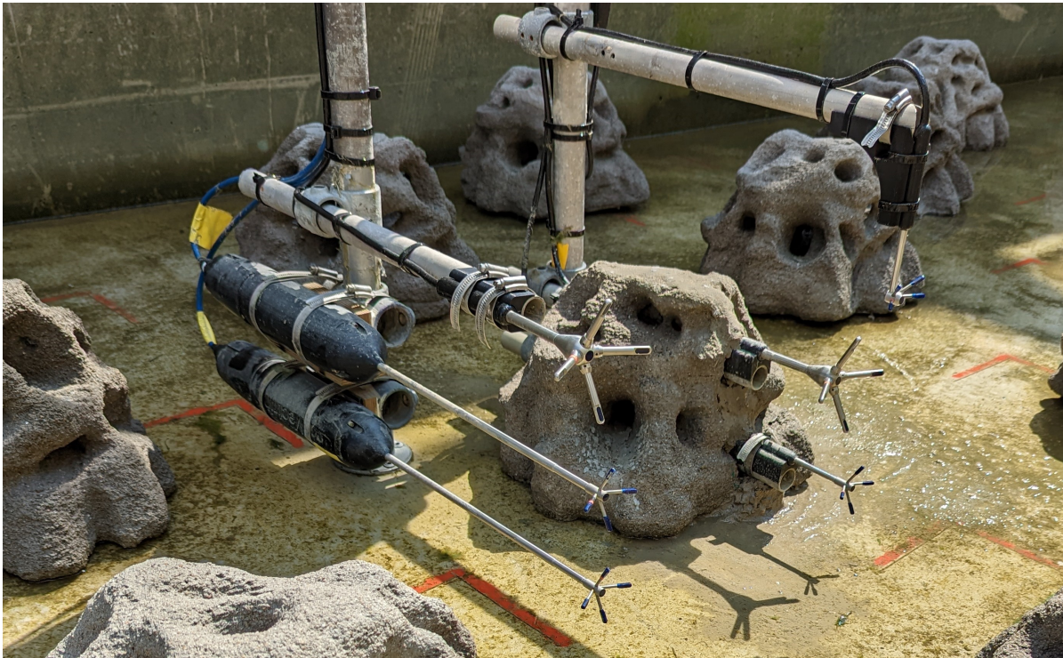
Figure 3.15: Picture of the actual ADV set up during testing.
