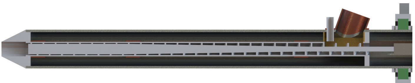
Fig 67: Crossection of the 3D extruder
