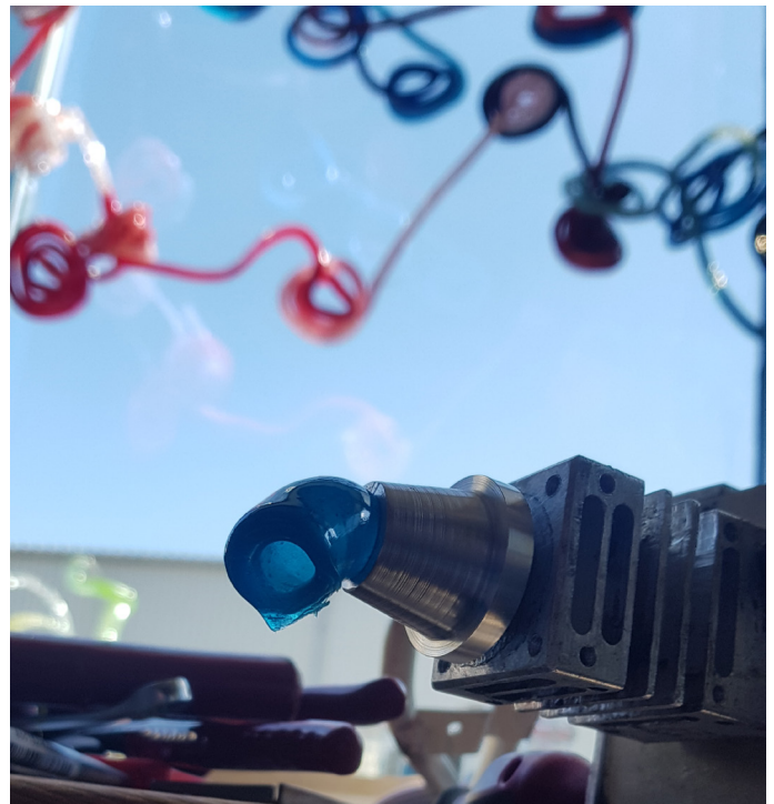
Fig 23: Extrusion with the nozzle with a core
