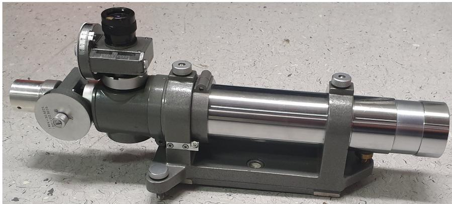
Figure 48: Autocollimator. Black ocular is used for measurement.
