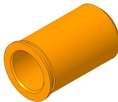
Figure 43: CAD representation of the M6 x 0.25 bushing from Thorlabs. [1]
