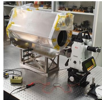
(c) Measuring LoS of the collimator.
