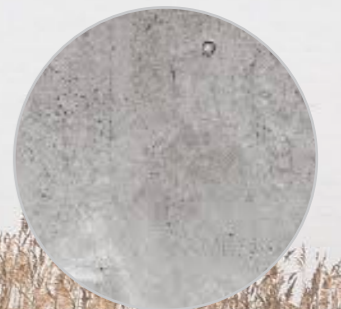
Semi-polished, rock salt finished precast concrete panels with aggregate from the Court of Appeals
