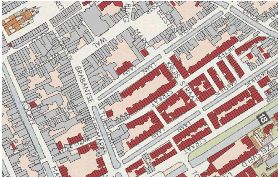
Figure 3.18: 2PM building footprints (dark red) and aligned building footprints (grey)
