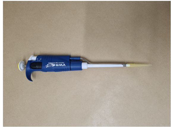
Figure A.4.: Precision Pipette used to place droplets of silicon oil.
