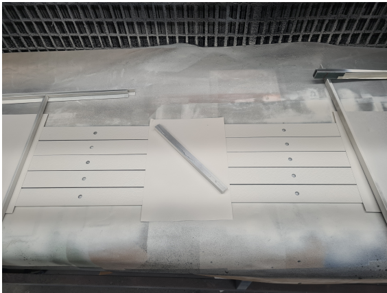
Figure 3.6.: Two-layer industrial-grade white paint coating.
