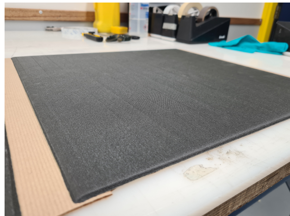
Figure A.9.: A textured, rough surface resulting from the peel-ply.
