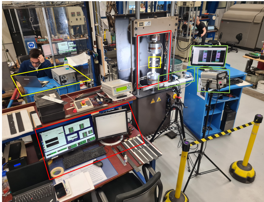
Figure 3.11.: Overview of experimental setup; Yellow: AE system. Green: DIC system. Red: MTS fatigue machine and control interface.
