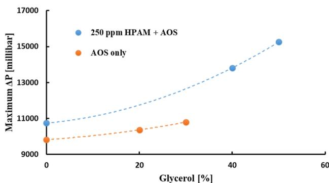
**Figure 13.** Comparison of the maximum pressure drop over the whole core length obtained for foam generated by solutions with and without the addition of 250 ppm HPAM. As it suggests, the AOS surfactant with 250 ppm HPAM significantly increases the pressure drop compared to the AOS surfactant solely, which leads to more stable foam in porous media.
