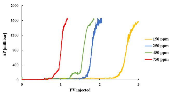
**Figure 17.** Pressure drop over the outlet section of the core vs the PV injected for foam is generated by a range of HPAM concentrations. The figure demonstrates that higher concentrations of HPAM reach higher pressure drop with fewer PV injected compared to lower concentrations.
