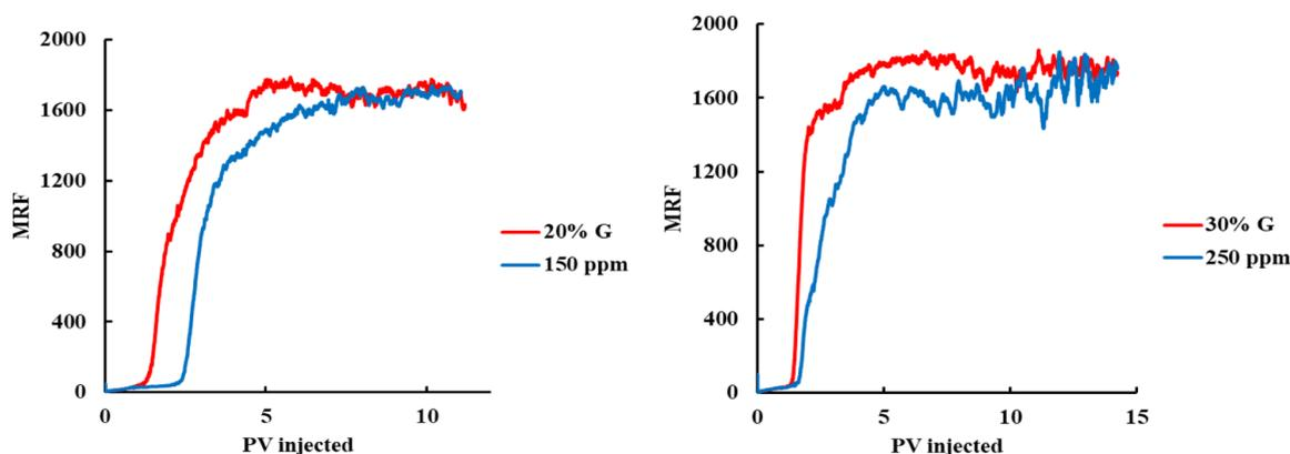
**Figure 20.** Comparison of the MRF vs PV injected of pair 1 (left) and pair 2 (right). As the figure suggests, both the pairs reached the similar MRF after several injections. However, in both cases, glycerol reached stronger foam faster than HPAM.
