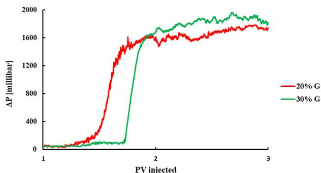
**Figure 16.** Pressure drop over the outlet section of the core vs the PV injected for a foam generated by 20 and 30% glycerol solutions. It indicates a trend that an increase in the glycerol concentration leads to a delay in the generation of a strong foam at the outlet section.
