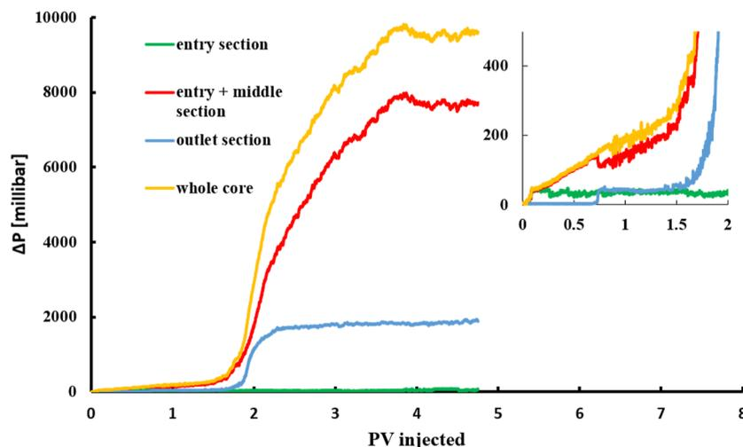
**Figure 8.** Sectional pressure drops for the control experiment vs the PV injected. The figure suggests that in the entry section, no significant pressure drop is observed. However, in the other section till 2 PV injection, a notable pressure drop is observed.
