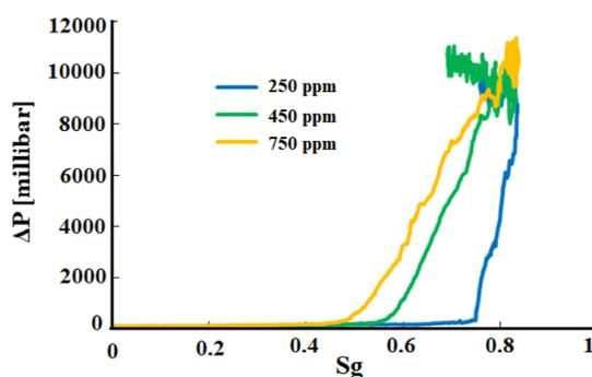
**Figure 22.** Pressure drop over the whole core vs the gas fraction inside the core for foam generated by 250, 450, and 750 ppm HPAM. As the figure suggests, higher concentrations of HPAM could generate strong foam at lower  $S_g$  compared to lower concentrations.
