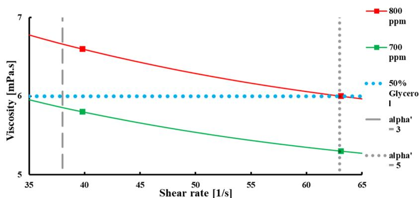
**Figure 7.** Matching of the apparent viscosity of the 50% glycerol solution with that of HPAM solutions. As the figure indicates, at 50% glycerol, parameter  $\alpha'$  has a significant effect on apparent viscosity, and more shear thinning can be observed.
