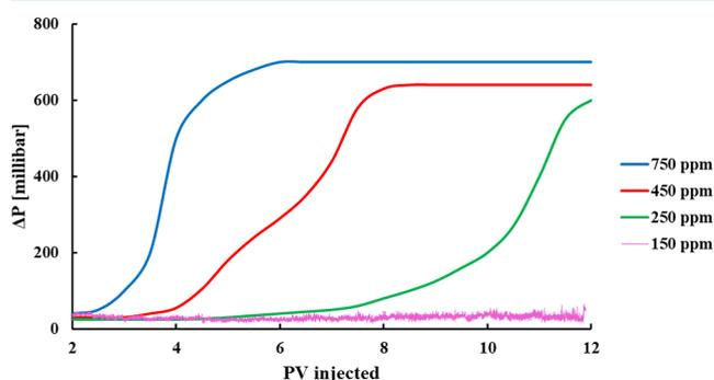
**Figure 14.** Pressure drop over the entry section of the core vs the PV injected for a foam generated by a range of HPAM concentrations.
