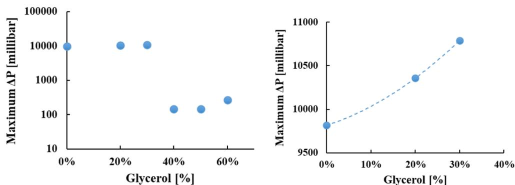
**Figure 10.** Maximum pressure drop over the whole core length was obtained for all glycerol experiments (left) and for the experiments containing up to 30% glycerol (right). For concentrations above 40% of glycerol, pressure drop decreases significantly compared to that for lower concentrations. However, for concentrations lower than 30%, by increasing the glycerol concentration, the pressure drop increases.
