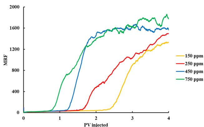
**Figure 19.** MRF over the whole core vs the PV injected for foam generated by a range of HPAM concentrations. As the figure indicates, since the equilibrium is reached much later in the inlet section and a bit later in the outlet section, the assumption is made that the strong foam starts to develop in the midsection, propagates toward the outlet section, and then propagates back toward the inlet section.
