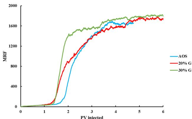
**Figure 18.** MRF over the whole core vs the PV injected for foam generated by solutions containing 0, 20, and 30% glycerol. According to the figure, the pressure development starts after injection of 1.4 PV, while for the outlet section, the pressure drop starts to increase for 1.5 PV and 1.8 PV. This points to the start of the generation of strong foam occurring in the section before the outlet section and propagating toward the outlet section.
