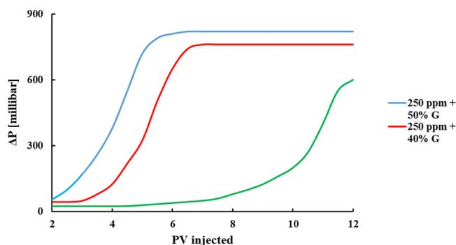
**Figure 15.** Pressure drop over the entry section of the core vs the PV injected for foam generated by a 250 ppm HPAM solution with and without glycerol. As the result indicates, pressure drop over the entry section by adding glycerol increases tremendously compared to that caused by 250 ppm HPAM alone.
