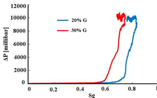
**Figure 23.** Pressure drop over the whole core vs the gas fraction inside the core for foam generated by 20 and 30% glycerol. It indicates a trend that an increase in the glycerol concentration leads to generation of a strong foam at lower  $S_g$ .
