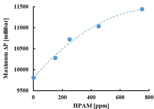
**Figure 11.** Maximum pressure drop over the whole core length obtained for all HPAM experiments. It indicates that by increasing the HPAM concentration, its pressure drop also increases, which is not similar to the glycerol trend.
