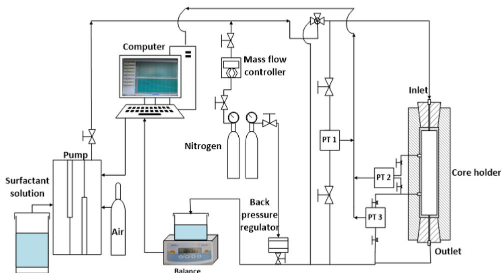
**Figure 2.** Setup used in the core flooding experiments.
