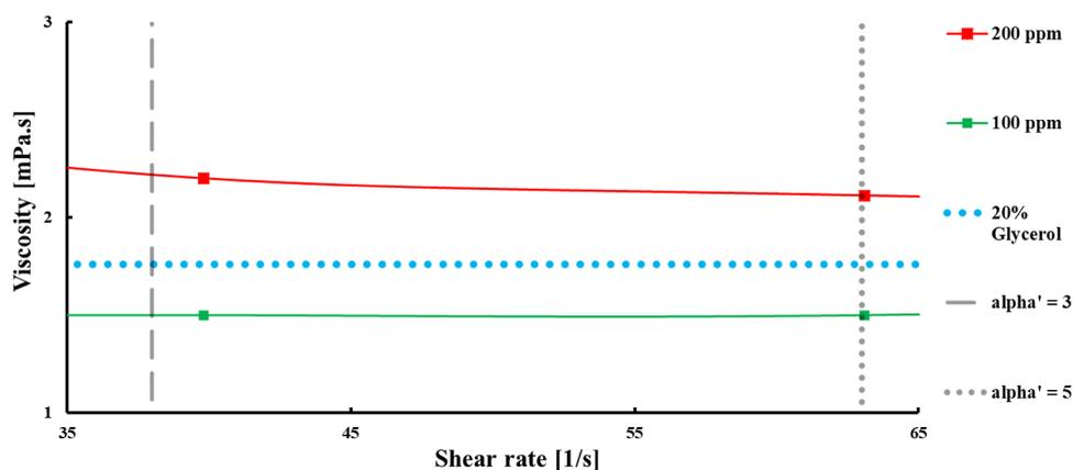
**Figure 6.** Matching of the apparent viscosity of the 20% glycerol solution with that of HPAM solutions. As it suggests, parameter  $\alpha'$  has no effect on the apparent viscosity in this domain, and no shear thinning can be observed.
