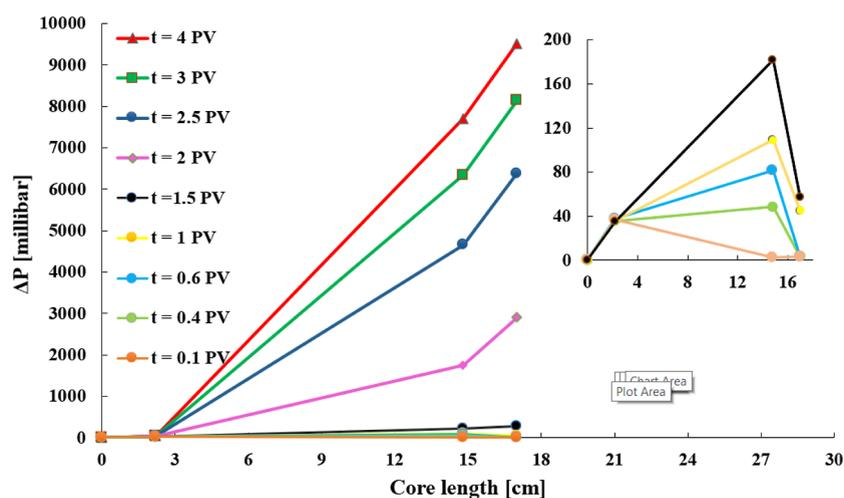
**Figure 9.** Sectional pressure drop vs the core length, for two different foam regimes. First, the foam propagates from the inlet toward the outlet (onset), after which the pressure drop increases drastically starting at the outlet (inset).
