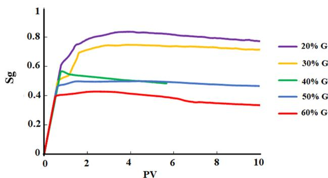
**Figure 21.** Gas fraction inside the core vs the PV injected for foam generated by a range of glycerol concentrations. According to the result, solutions with higher glycerol concentrations have less  $S_g$  compared to those with lower concentrations of glycerol. It indicates that lower concentrations of glycerol are able to displace liquids in the core.
