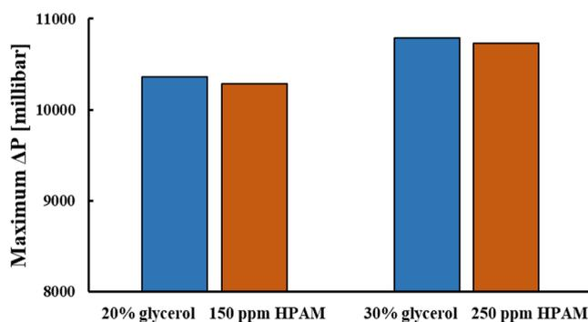
**Figure 12.** Comparison of the maximum pressure drop over the whole core length for the pairs of glycerol–HPAM. According to the figure, both Newtonian and non-Newtonian agents show similar pressure drop.
