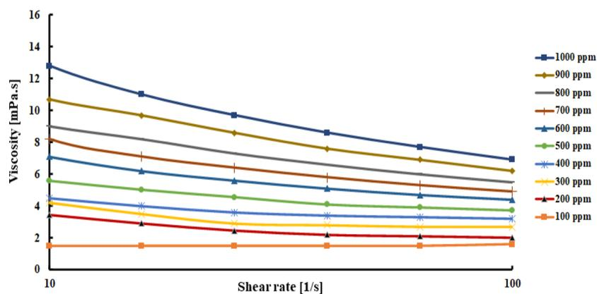
**Figure 4.** Measured apparent viscosity for a range of HPAM concentrations in the shear rate domain of [10/s to 100/s]. By increasing the shear rate, viscosity decreases. For higher concentrations, the decrease is higher compared to that at lower concentrations.
