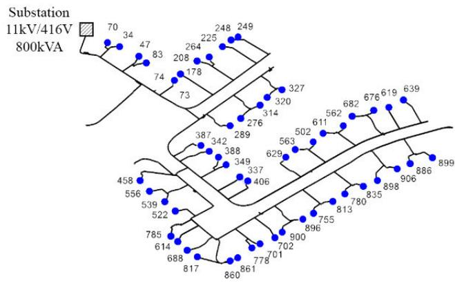
Figure 3.3: Single line diagram of the IEEE European low voltage feeder
