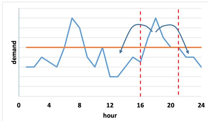
Figure 2.3: Example of load shifting,[7]
