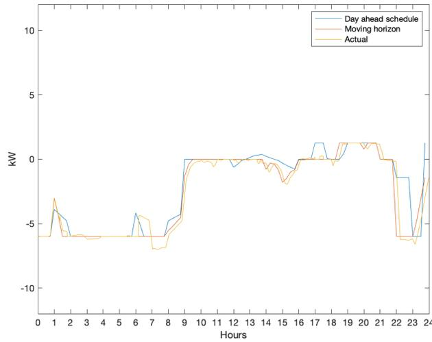
Figure 6.5: Grid exchange from different time frames
