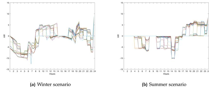
Figure 4.11: Grid power exchange from 55 households in the feeder (+ feeds, - draws)
