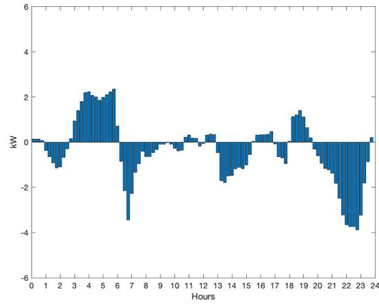
Figure 6.6: Grid power deviations due to forecast errors
