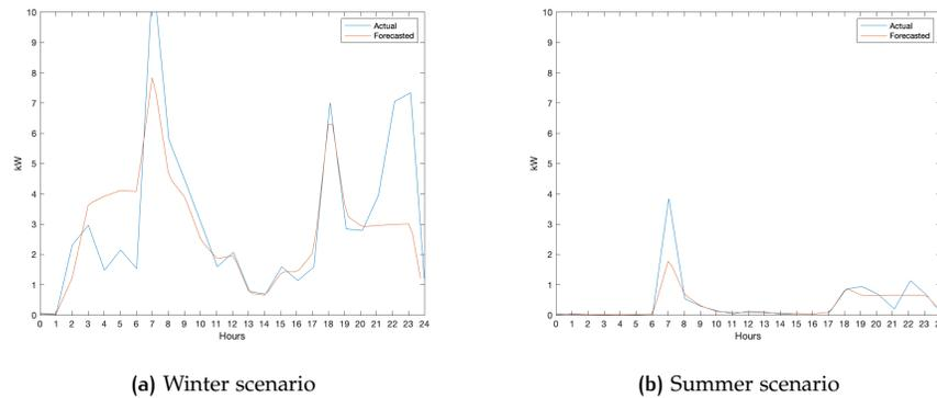
Figure 4.6: Actual and forecast heating profiles of tier 1
