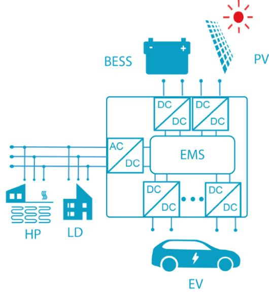
Figure 3.1: Smart energy system's diagram [56]
