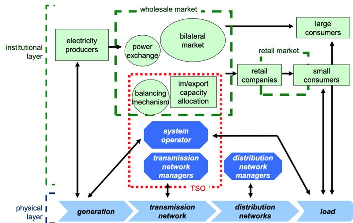
Figure 2.5: Diagram of electricity system,[27]
