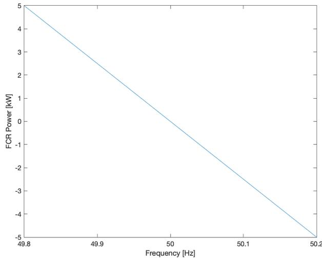
Figure 7.2: Droop corresponding to 5kW reserve capacity and 10kW nominal capacity
