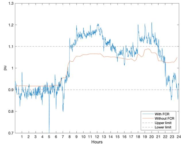
Figure 7.7: Voltage at BUS 906 in the feeder with FCR and without
