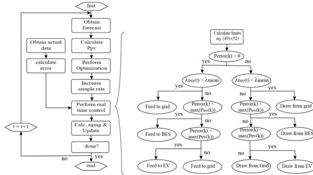
Figure 3.2: Moving horizon and real time control flowchart [56]
