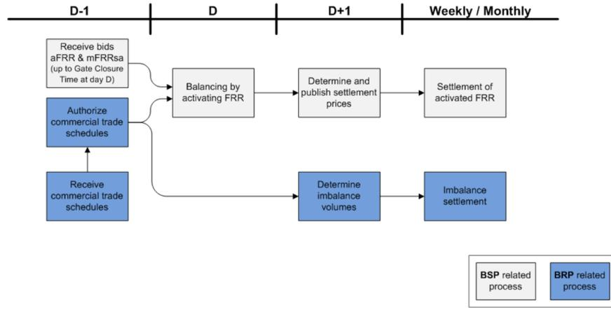
Figure 7.1: Balancing process diagram, [51]
