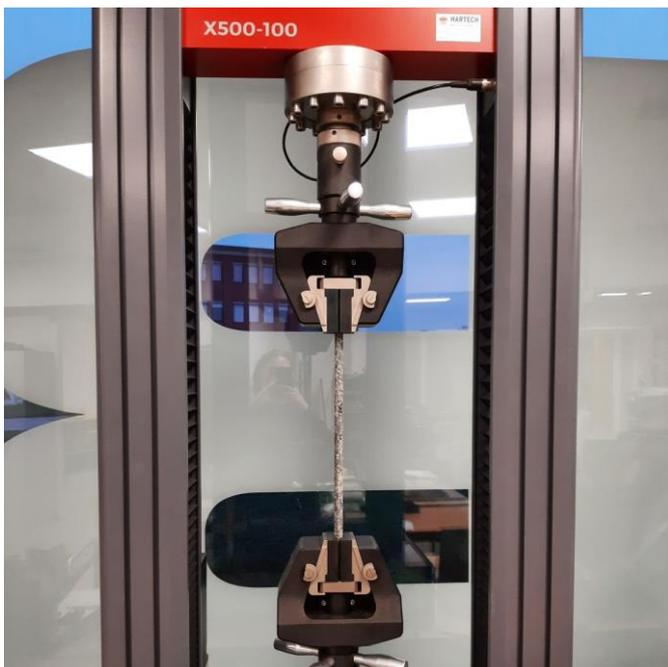
*Figure 0.39: Steel pulling test (source: Nebest)*
