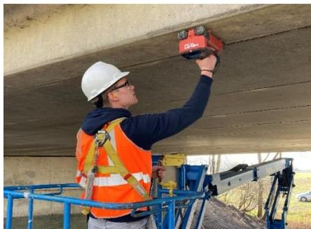
*Figure 0.30: Usage of a concrete radar (source: Nebest)*
