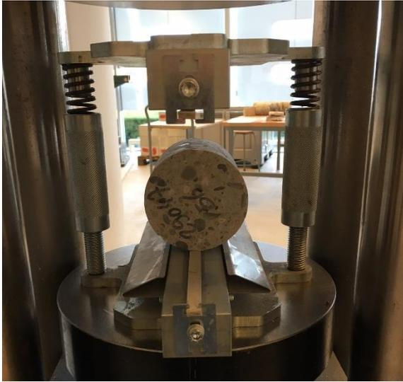
*Figure 0.37: Tensile splitting force test of concrete specimen (source: Nebest)*
