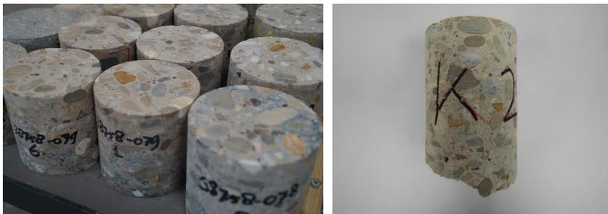
Figure 0.36: Concrete core specimens (source: Nebest)
