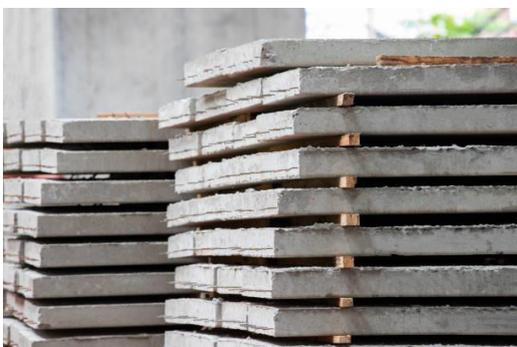
Figure 6.9: Storage of concrete elements (Ratchat, n.d. )
