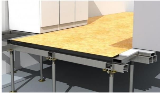
Figure 0.52: Computer floor (System floor technics, n.d.)
