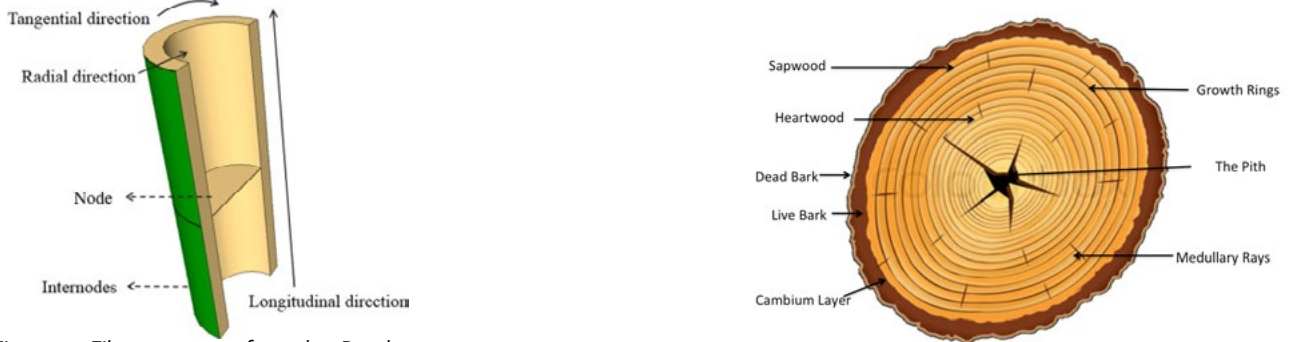
Figure 19: Fiber anatomy of wood vs Bamboo.
