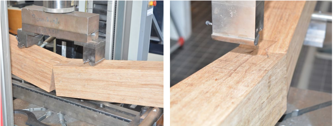
Figure 88: Images from four Point bending test
