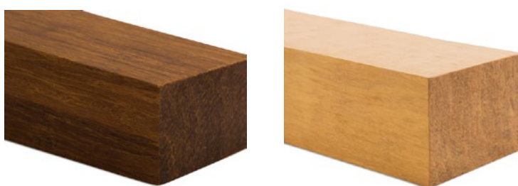
Figure 27: Strand laminated bamboo beam("eco friendly," n.d.)
