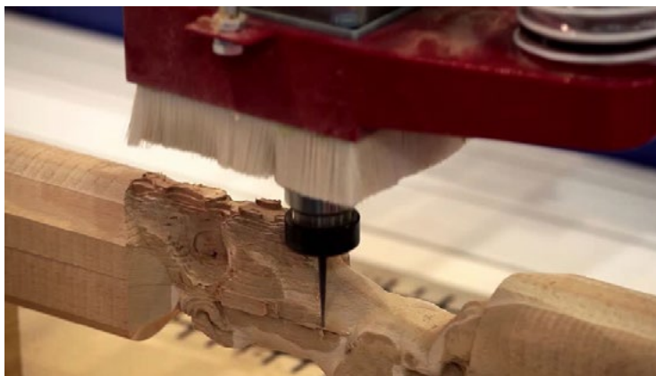
Image showing Wood CNC engraving and cutting machine close up processing
