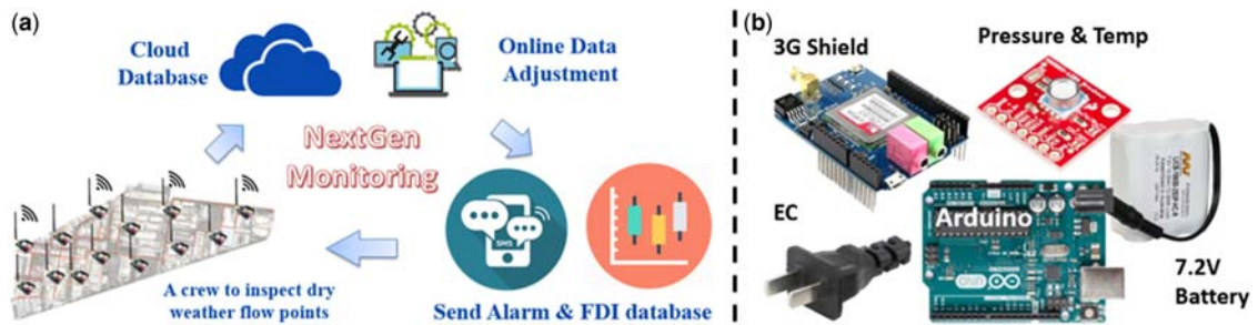
Figure 11.14 (a) data collection process of NextGen Urban Water Monitoring network; (b) Arduino logger package including cheap US power cable, 3G shield, MS5803 pressure sensor and 7.2 V battery. Source: EPHM Lab and BoSL.
