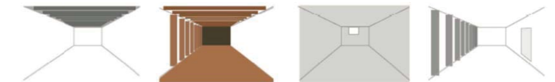
Image 3. Own illustration. Aspects that have influence on the appearance of the spatial boundaries, from left to right: depth/shadow, color/material, focal accents, breaks/disturbing objects.
