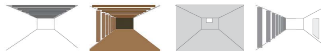
Image 4. Own illustration. Aspects that have influence on the appearance of the spatial boundaries, from left to right: depth/shadow, color/material, focal accents, breaks/disturbing objects.
