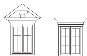
18 Wooden window framing Single glazing Masonry lintels
