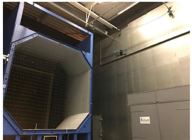
Fig. 1 Open jet facility, which is a large-scale wind tunnel, and the tested quadrotor.
