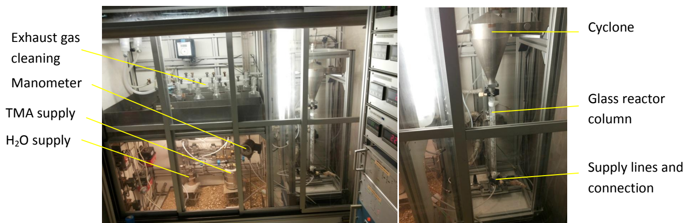
Figure 4.35: The ALD setup used in this experiment, showing the whole setup including bubblers and gas cleaning (left) and the reactor with connections (right).
