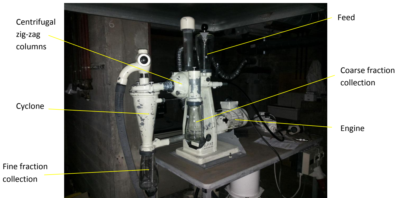
Figure 4.32: The Alpine 100 MRZ laboratory zig-zag classifier used for wind sifting and its different parts.
