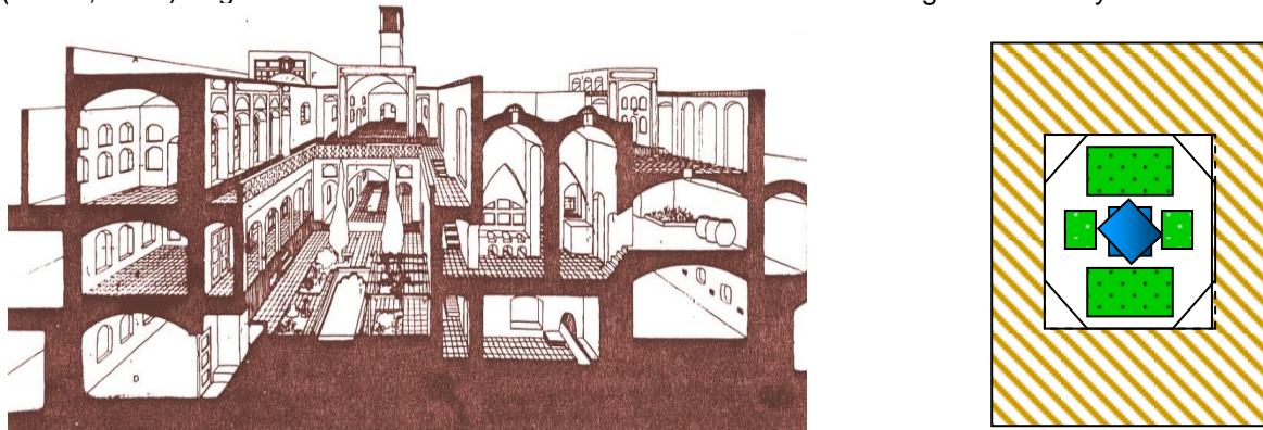
Figure 5.23. Cross-section of a house with a multi-storey courtyard (Tavasoli, 1989) with courtyards' scheme
