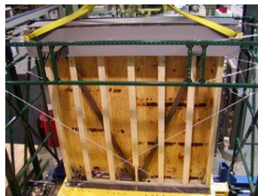
Figure 4.6 Damping system made of fluid-filled shock absorbers, installed horizontally throughout the walls to channel some of the energy into dampers (Photo: Rensselaer/Symans, 2006)
