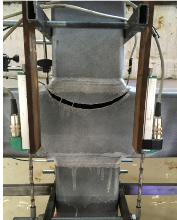
Figure 4.7: Chord side wall failure joint X8
