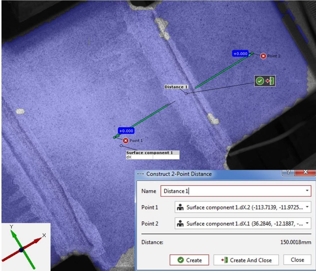
Figure 4.14: DIC data points for comparison to the 3% deformation limit
