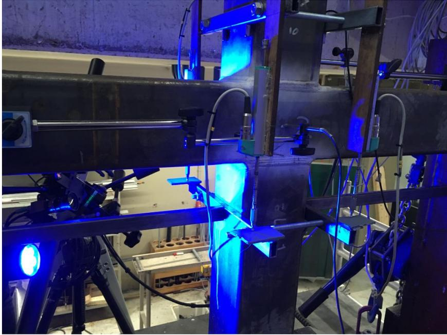
Figure 4.4: Positioning LVDTs on joint X2 during the experiment (1)
