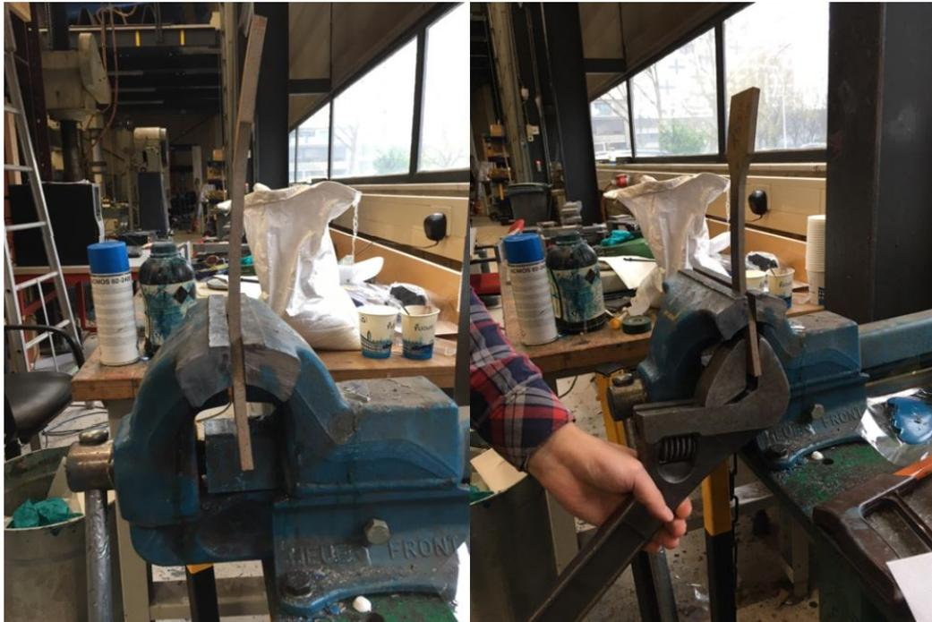
Figure 3.4: Bending of the coupon grip section
