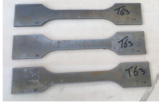
Figure 3.2: Coupon specimens T63-series
