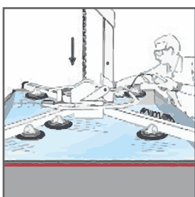
Placement of glass on frame.
