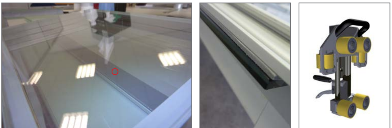
Figure 7.1.6 - Minor air encapsulation which are rarely visible. Wider tape will give more risk on air encapsulation. First application of the tape on glass, decreases the chance on visible air encapsulation. Right picture is a hand presser with pressure indicator (own ill.)
