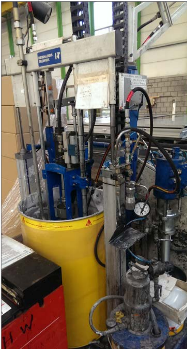
Figure 2.3.1 - 2-component mixer at Scheldebouw. (Own ill.)
