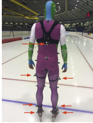
(a) IMU sensors on skaters body [43].
