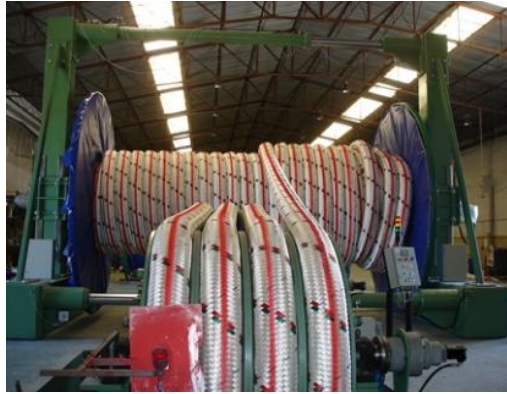
FIGURE 52: MOORING FIBRE ROPE (LANKHORST ROPE 2012)
