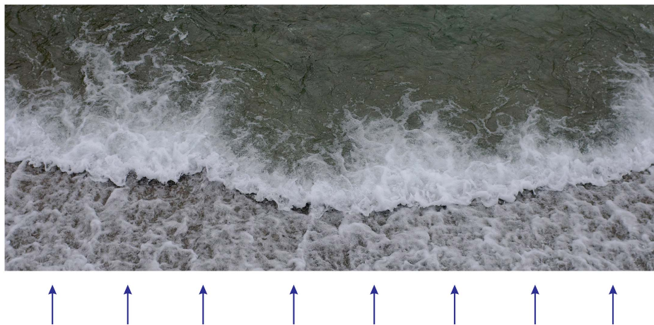
Fig. 1. Three-dimensional air–water surface features in a hydraulic jump along Katashima River, Japan, in October 2012 (shutter speed: 1/250 s). Arrows point in the inflow direction. (Image by Hubert Chanson.)
