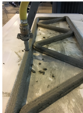
(b) Printing with a circular nozzle, from [12].
