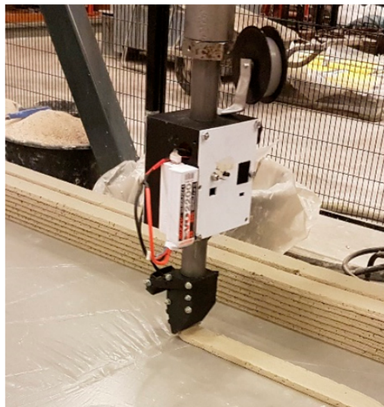
Figure 2.13: Entrainment of reinforcement cable in concrete filament during printing, from [37].
