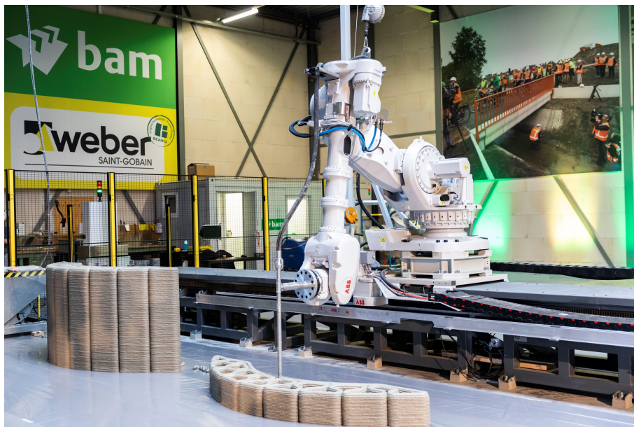
Figure 2.1: 3D concrete printing facility BAM Infra and SG Weber Beamix, from [6].
