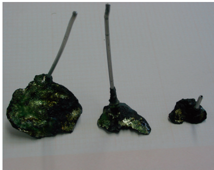
Figure 4.9: Examples of freezing of the steel meniscus using powder A2 and EMBr setting of 360 A
