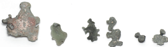
Figure 5.10: Slag fragments, “droplets”, sampled from inside the mould (approx. 50 cm depth) - Mould powder A
