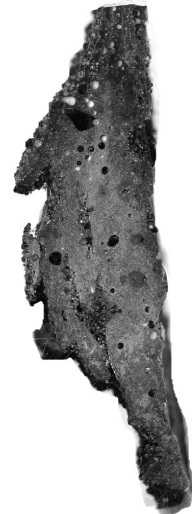
Figure 6.8: Slag rim, extracted from the mould - Mould powder M, thin slab caster. Right: mould side
