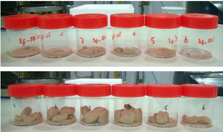
Figure 5-10. Dried cemented sand - (upper) after the treatment with high concentration; (lower) after the treatment with low concentration.
