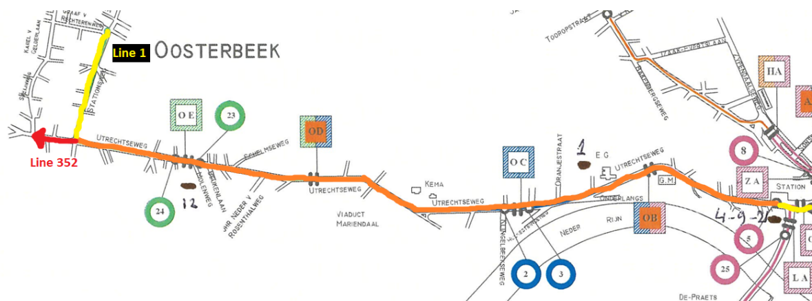
Figure 5.3: Part of the substation and feed-in section map that shows the route that line 352 follows. Its terminus is at section 5 at Arnhem CS and it goes West along all purple, blue and green sections.
