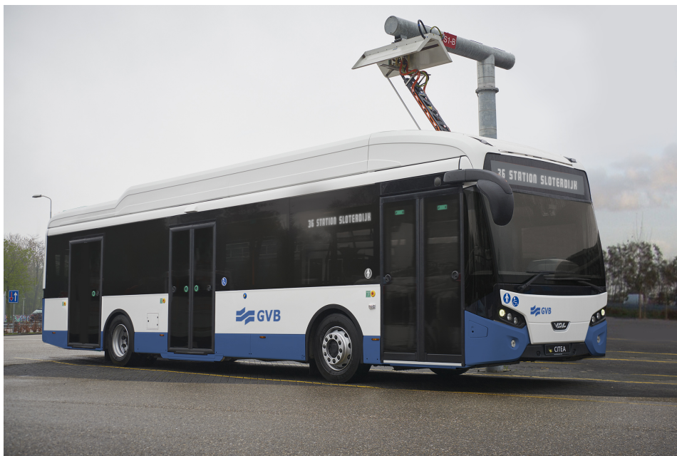
Figure 1.1: An e-bus with on-board battery. It is connected to the grid with its pantograph in order to charge the battery. It has to remain stationary in order to charge. [1]
