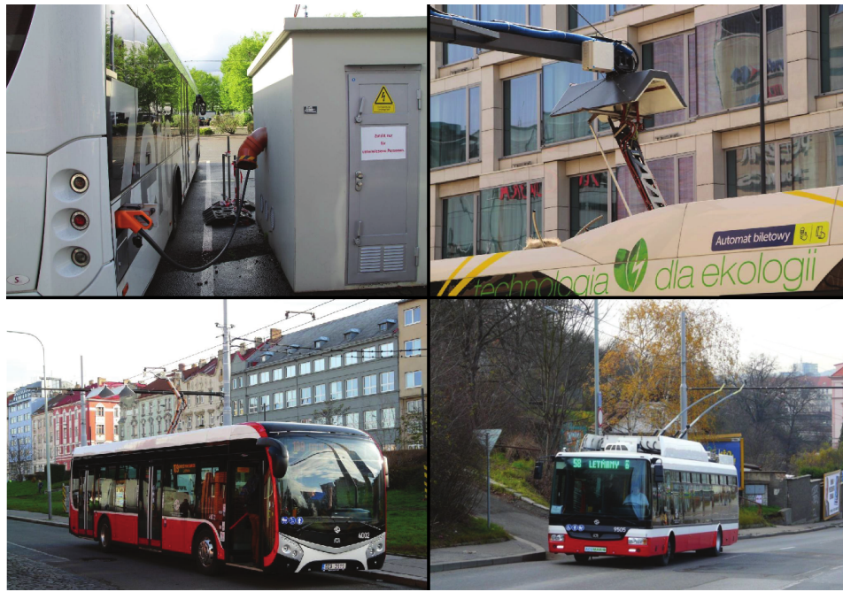
Figure 1.3: Examples of different charging methods. (Top left) Plug-in connectors are typically used for overnight charging. (Top right) Four-pole systems are typically used for fast/opportunity charging. (Bottom left) Two-pole systems are typically used for low to medium charging speeds. (Bottom right) A regular trolleybus connected to the grid. With the right internal adjustments (i.e. adding a traction battery) trolleybuses can be converted to IMC buses. [9]
