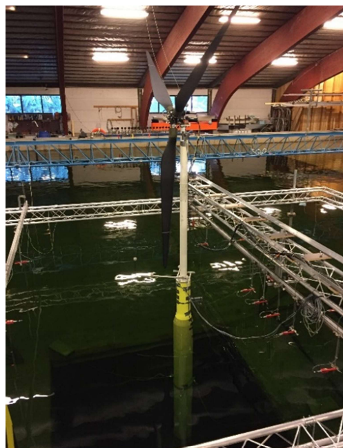
Figure 1. Impression of the scaled spar-buoy wind turbine layout used during the Hydralab+ tests.
