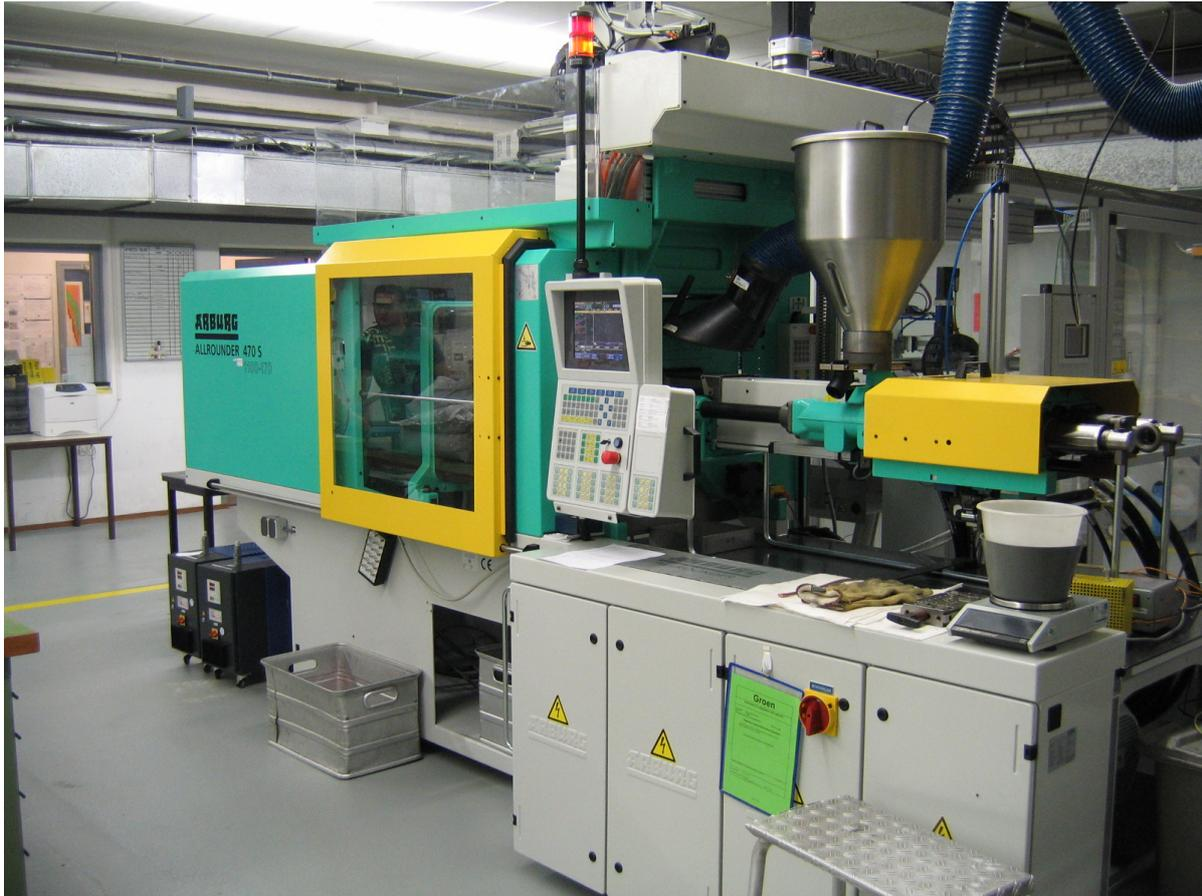
Figure 1.3: an injection molding machine.
