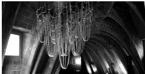
Figure 2.22: The hanging chain applied for 'Form Finding'
