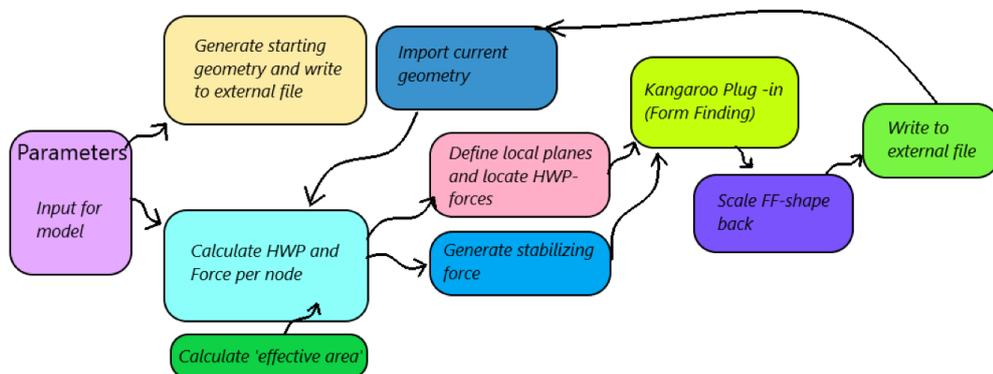
Figure A.9: A complete overview of the water pressure model in GH.
