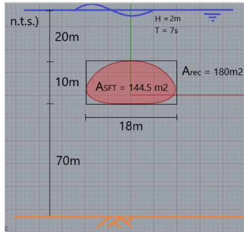
Figure 4.20: The situation for which the order of magnitude of the wave load is determined.
