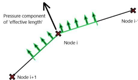
Figure B.3: The visualization of the pressure component of the 'effective length' per node
