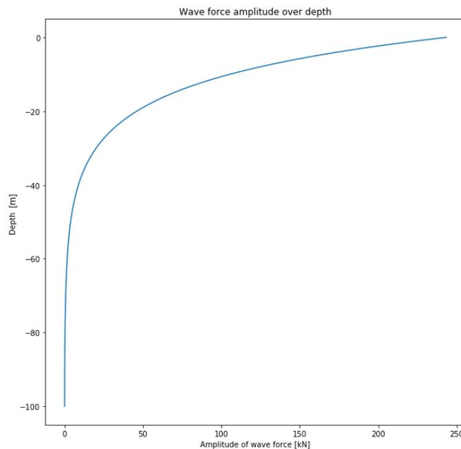
Figure 4.23: The amplitude of the wave force on the SFT vs depth
