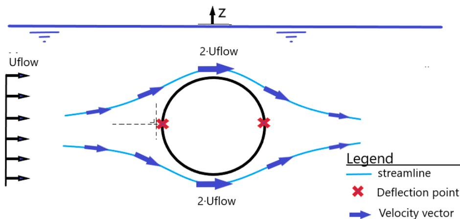
Figure 4.2: The velocity profile of a circular tube in a flow
