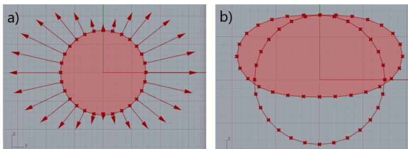
Figure B.4: The load profile and Kangaroo's output for the hydrodynamic current
