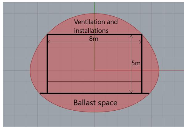
Figure 6.3: The optimal cross-section with use of internal space
