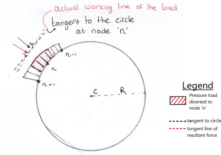
Figure 3.3: The tilted force due to non-uniform pressures
