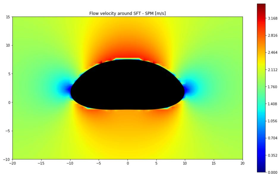
Figure 4.12: The flow velocity contour plot along SFT with geometry factor 5.0
