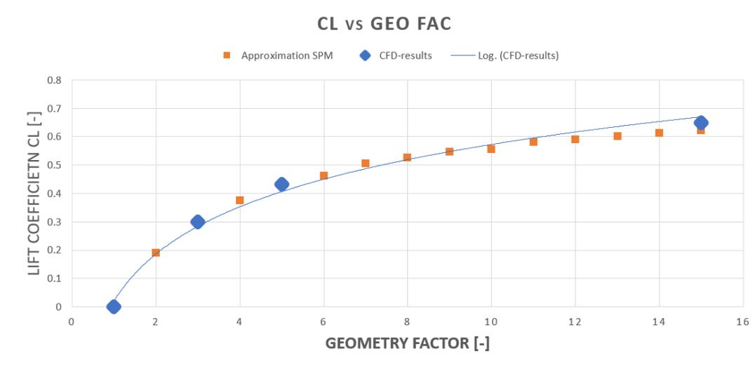
Figure 4.16: The relation between  $C_L$  and the Geometry Factor
