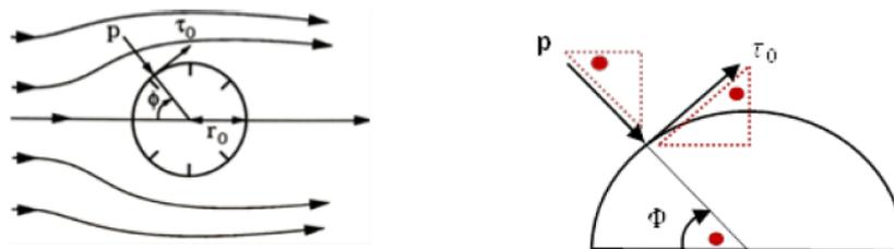
Figure 2.14: The forces perpendicular and parallel to a body [38].
