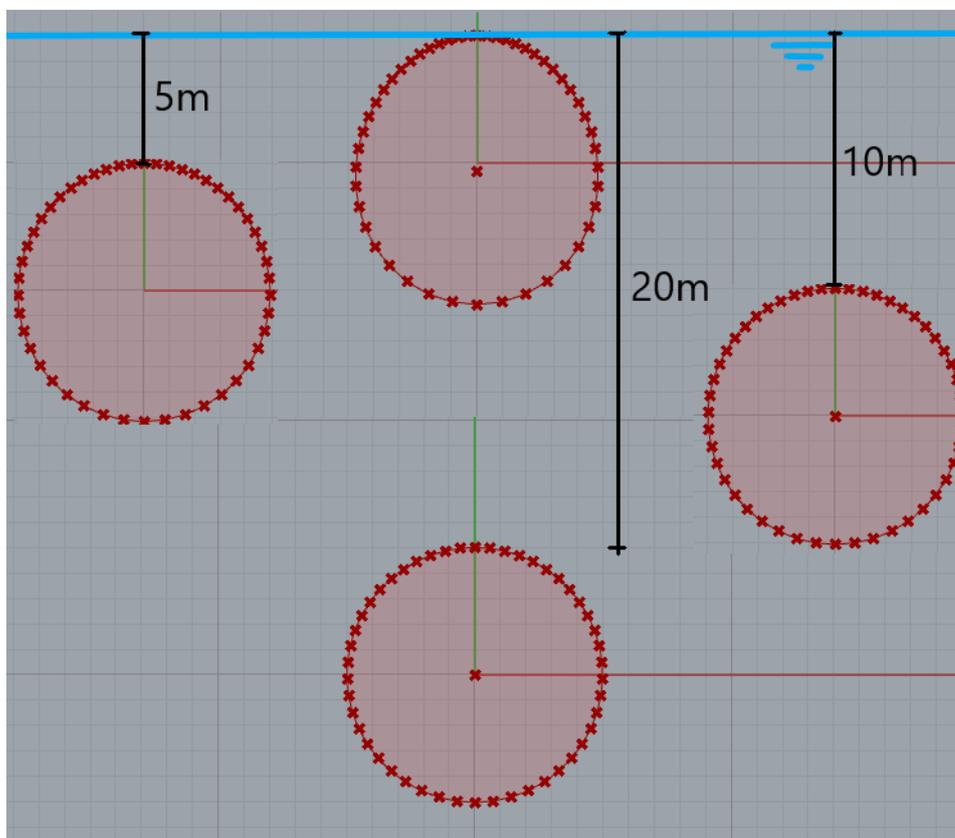
Figure 3.14: The optimal shape according to FF per depth
