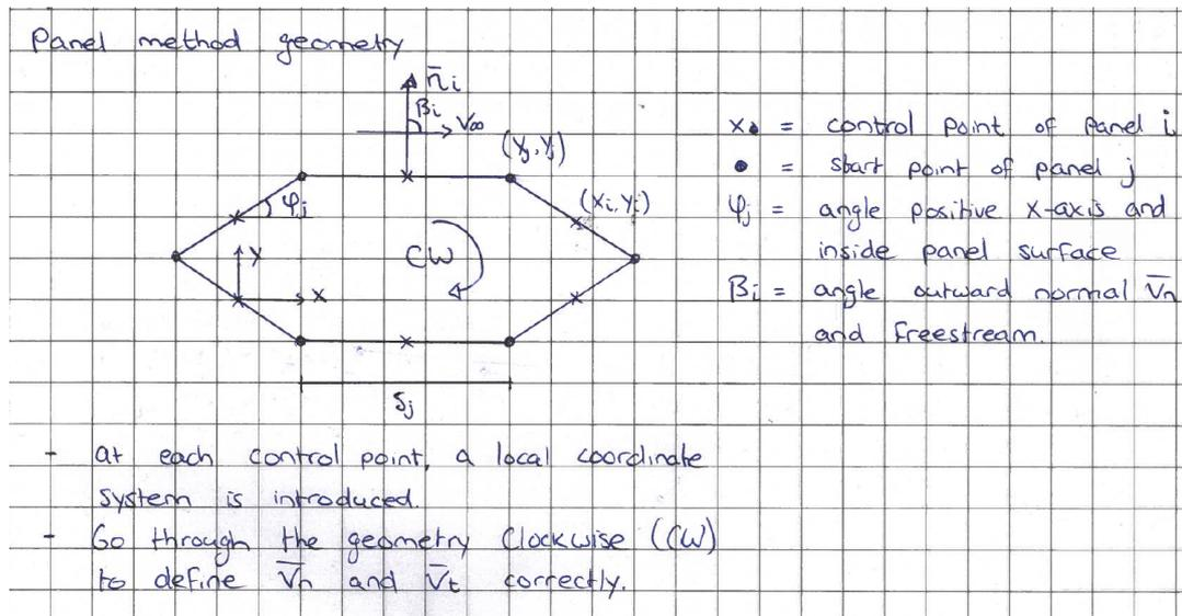
Figure E.2: The geometry definitions during the derivation
