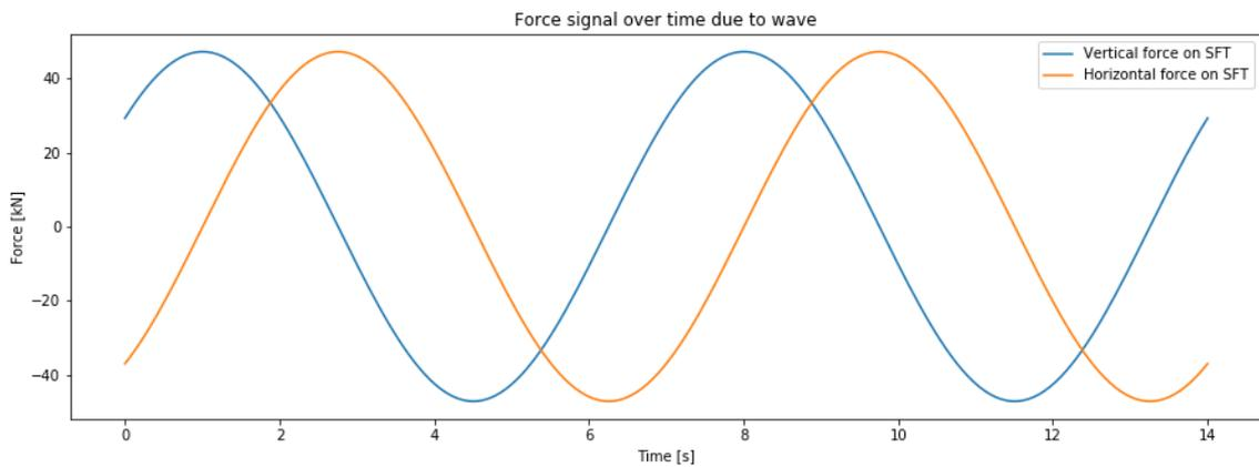
Figure 4.22: The wave load on the SFT according to LWT at 20m depth
