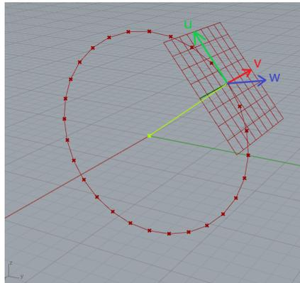
Figure 3.2: A locally generated plane, tangential to the circle
