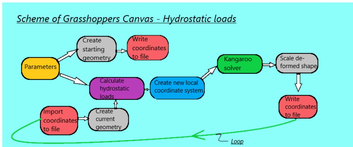
Figure 3.7: the external looping process in Grasshopper.
