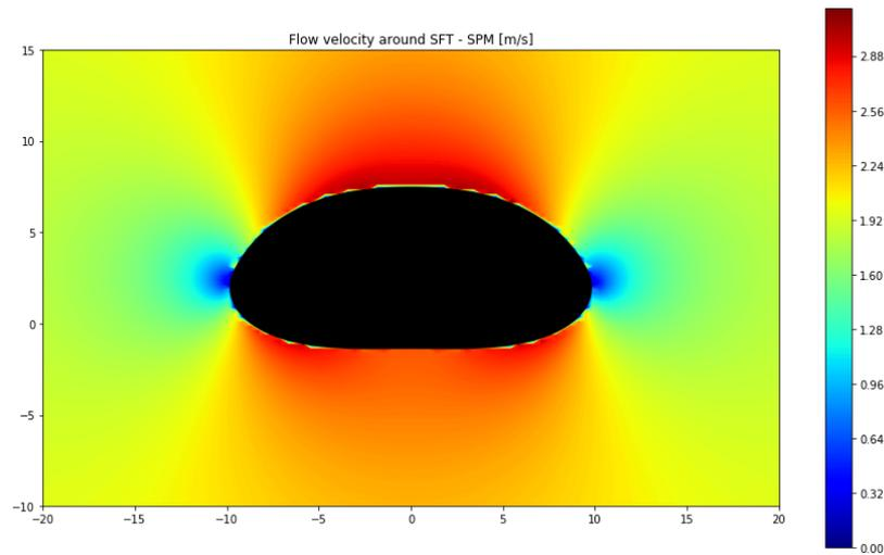
Figure G.3: The flow velocity profile for cross-section with GF = 3.0
