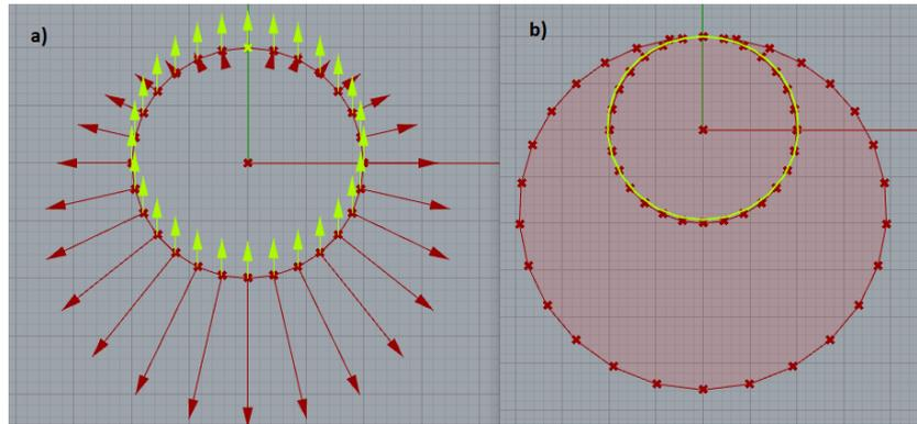
Figure A.6: a) the geometry with loads, vertical stabilization loads in yellow. b) the form-found shape, scaled back in yellow
