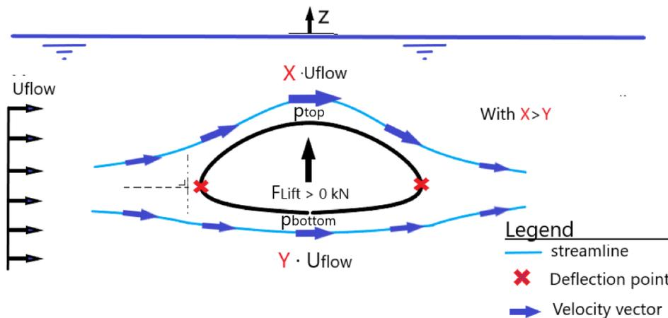
Figure 4.7: A sketch of the flow profile along the newly found cross-section
