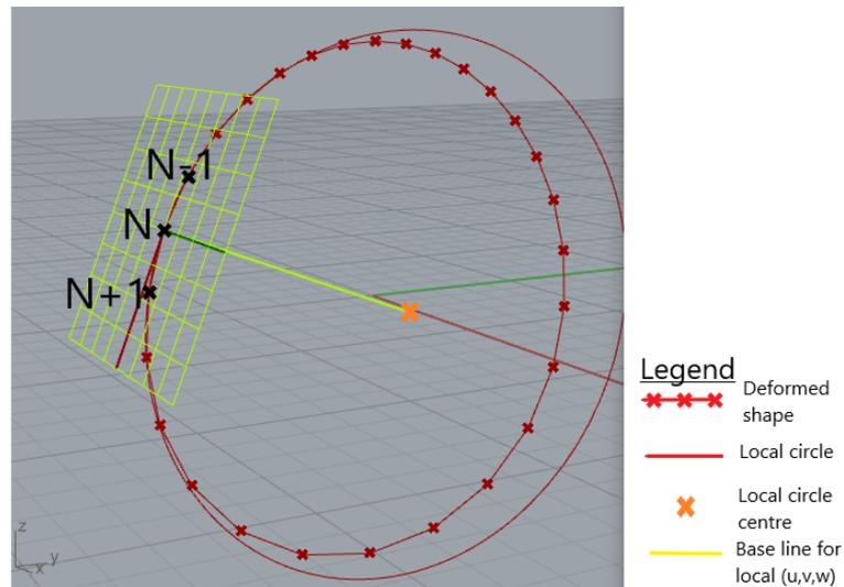
Figure 3.6: the underlying elements to help generating the new u,v,w, coordinate system.
