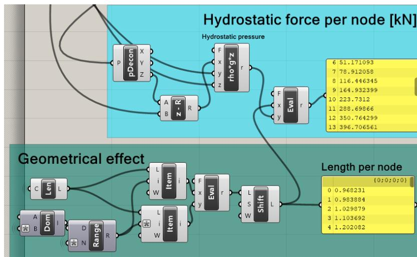
Figure A.2: The script in GH for the generation of the hydrostatic loads
