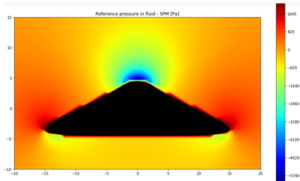
Figure 5.8: Pressure field - Panel Method
