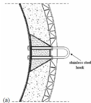
Figure 2.10: The attachment of the tethers to the SFT [29]
