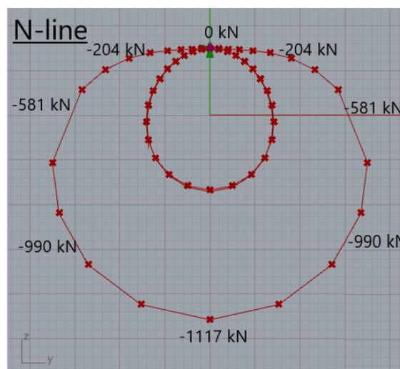
Figure 3.13: The N-line in the CS for the deformed shape
