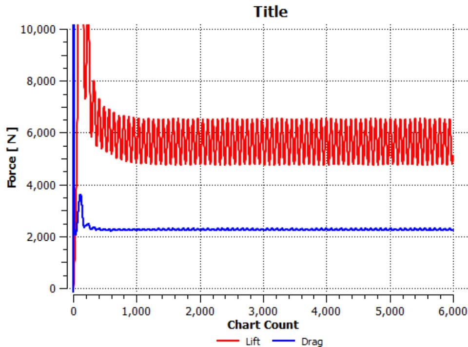
Figure G.6: The drag and lift force for cross-section with GF = 3.0 and  $V_\infty = 2 \text{ m/s}$  [43]
