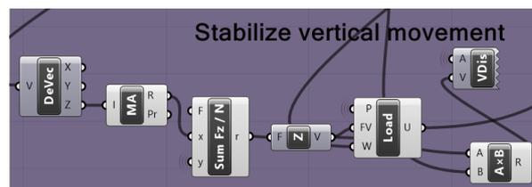
Figure A.7: The stabilizing force in GH's script
