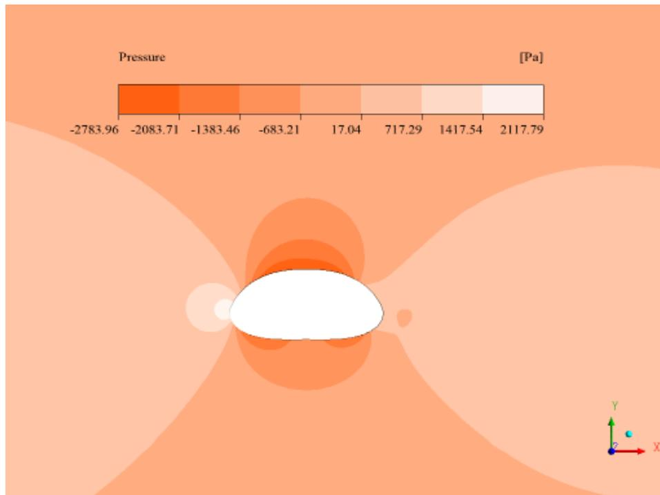
Figure G.5: The pressure field for cross-section with GF = 3.0 and  $V_\infty = 2 \text{ m/s}$  [43]
