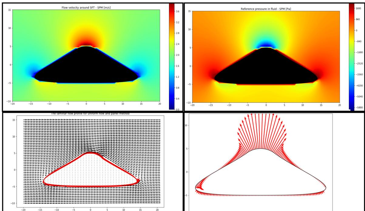
Figure F.11: Output of Python script - with exoskeleton and xFoil analysis
