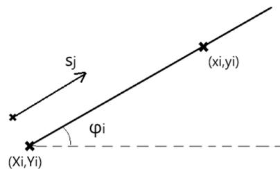
Figure E.4: The definition of  $x_i$  and  $y_i$  along panel length  $s_j$
