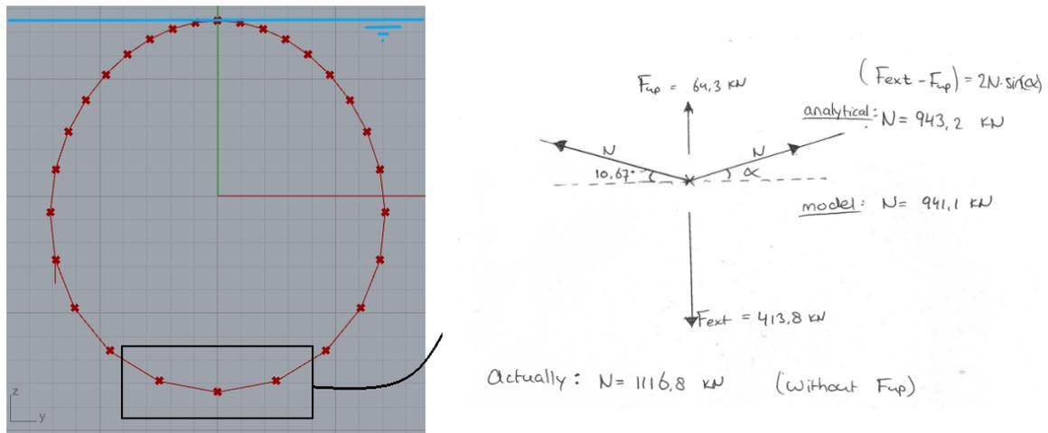
Figure 3.10: The equilibrium of the lowest node for the deformed shape
