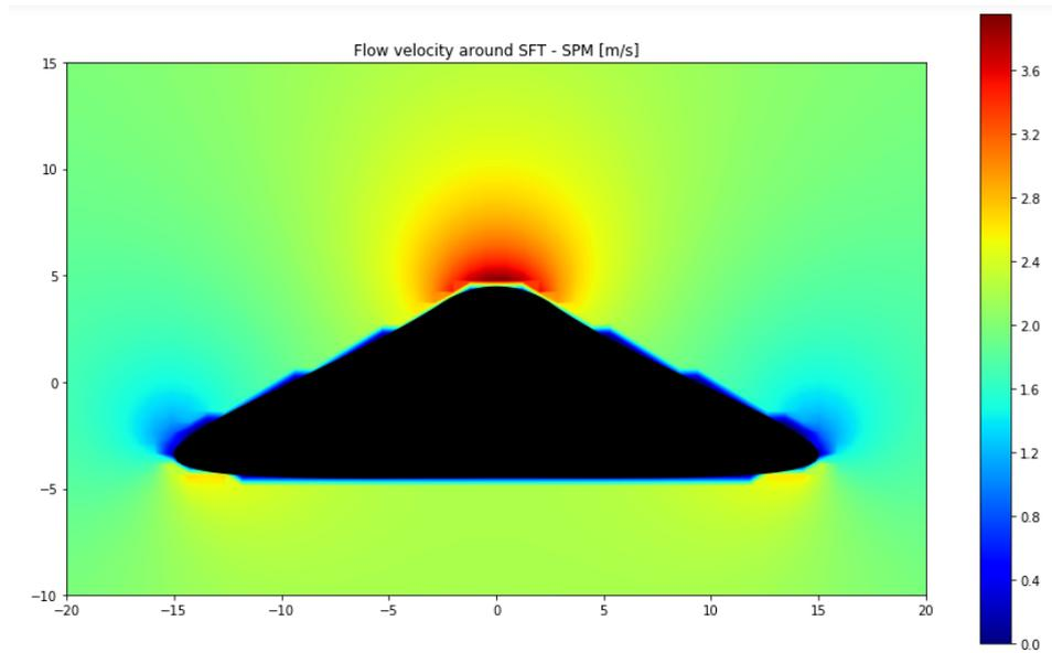
Figure 5.7: Velocity field - Panel Method
