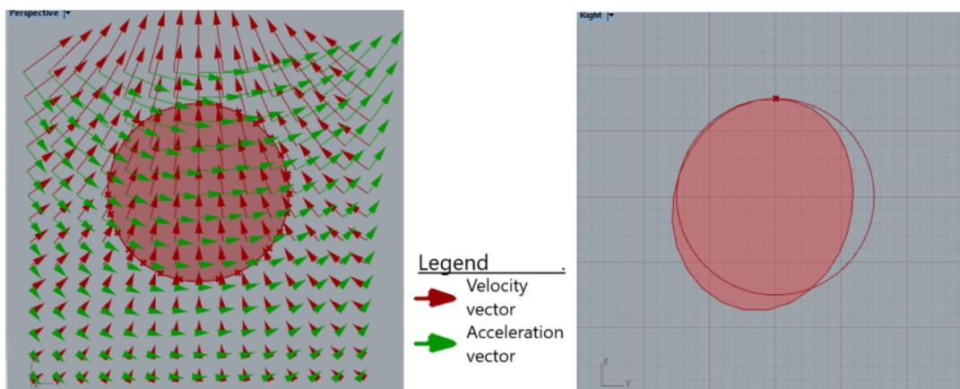
Figure 4.18: a) The starting geometry including load profile vectors, b) The FF-shape due to the load profile
