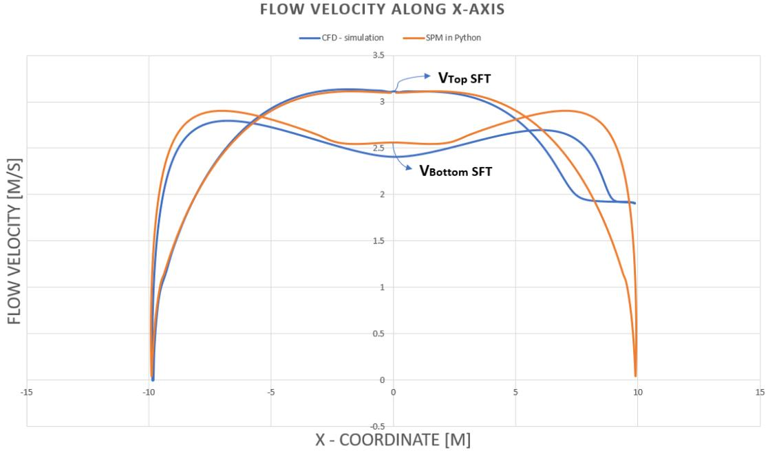
Figure 4.14: The velocity profile along the SFT for SPM and CFD-model
