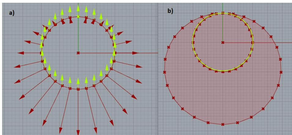
Figure 3.4: a) the geometry with loads, vertical stabilization loads in yellow. b) the form-found shape, scaled back in yellow
