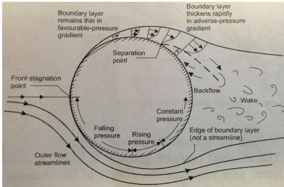
Figure 2.12: The turbulent flow around a submerged body [17]
