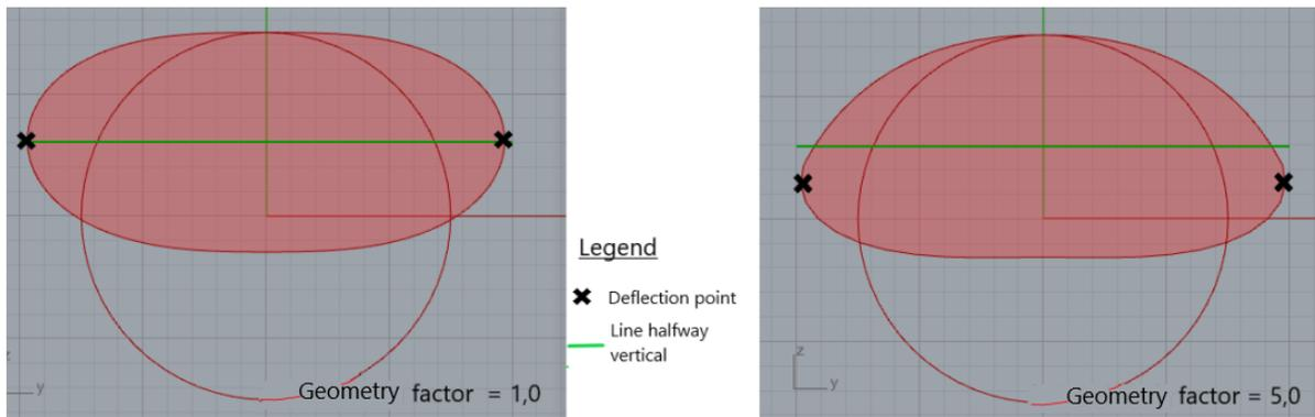
Figure 4.6: The deformed shapes from FF with amplification factors 1.0 (left) and 5.0 (right)
