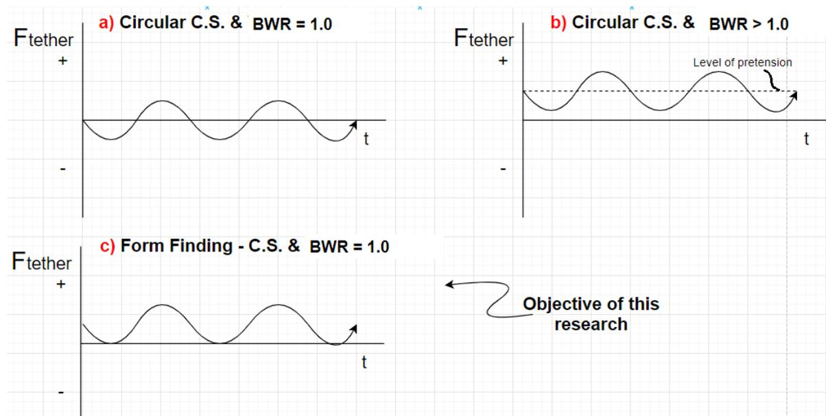
Figure 2.20: The forces in the tethers for different situations over time.
