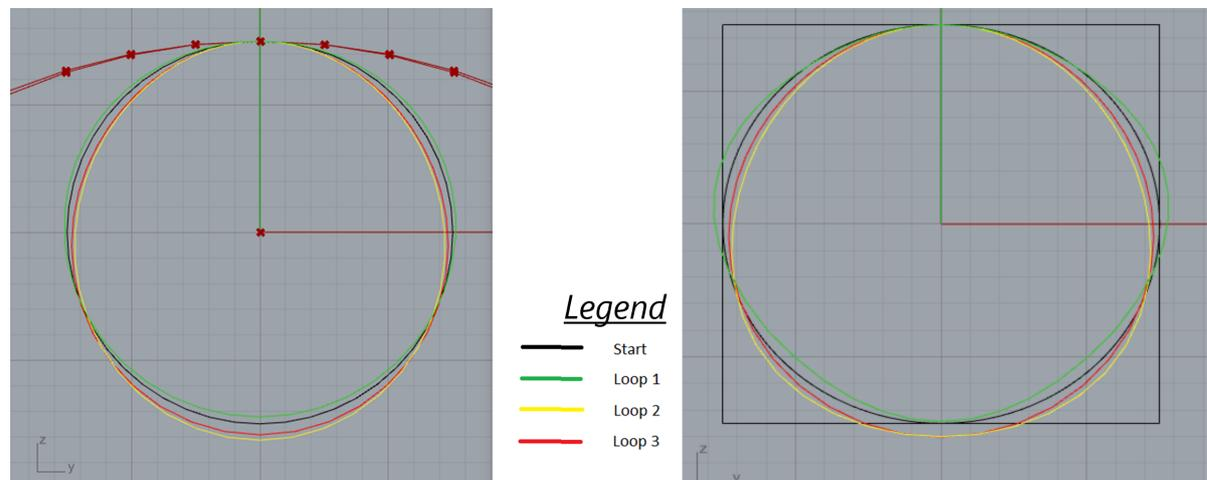
Figure A.12: The looping process with 3 loops for a circle (left) and a rectangle (right) as starting geometry
