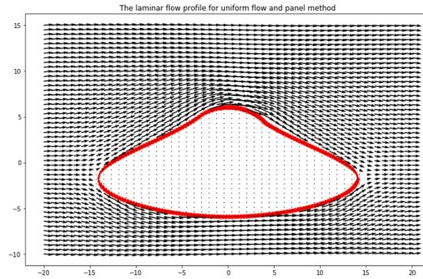
Figure 6.7: The composite cross-section and its flow profile
