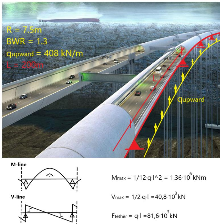
Figure 2.21: Sketch showing the presence of shear and bending for  $BWR \neq 1.0$ .
