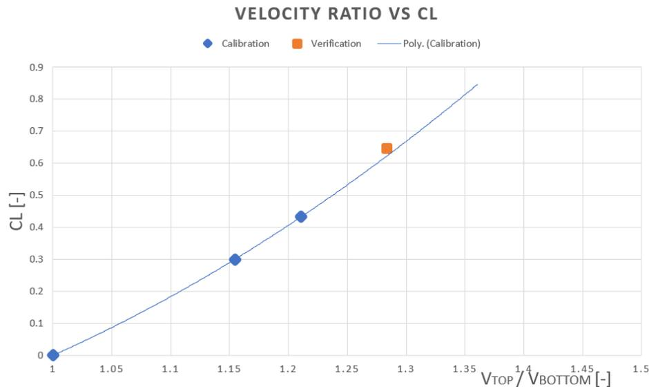
Figure 4.15: The relation between  $\frac{V_{top}}{V_{bottom}}$  and  $C_L$
