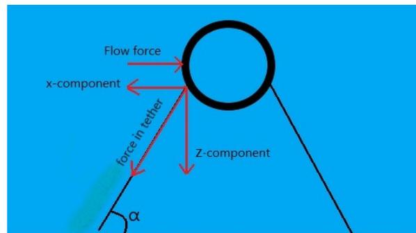
Figure 2.3: Horizontal capacity of tether under an angle
