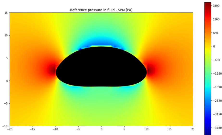
Figure 4.13: The pressure distribution contour plot along SFT with geometry factor 5.0
