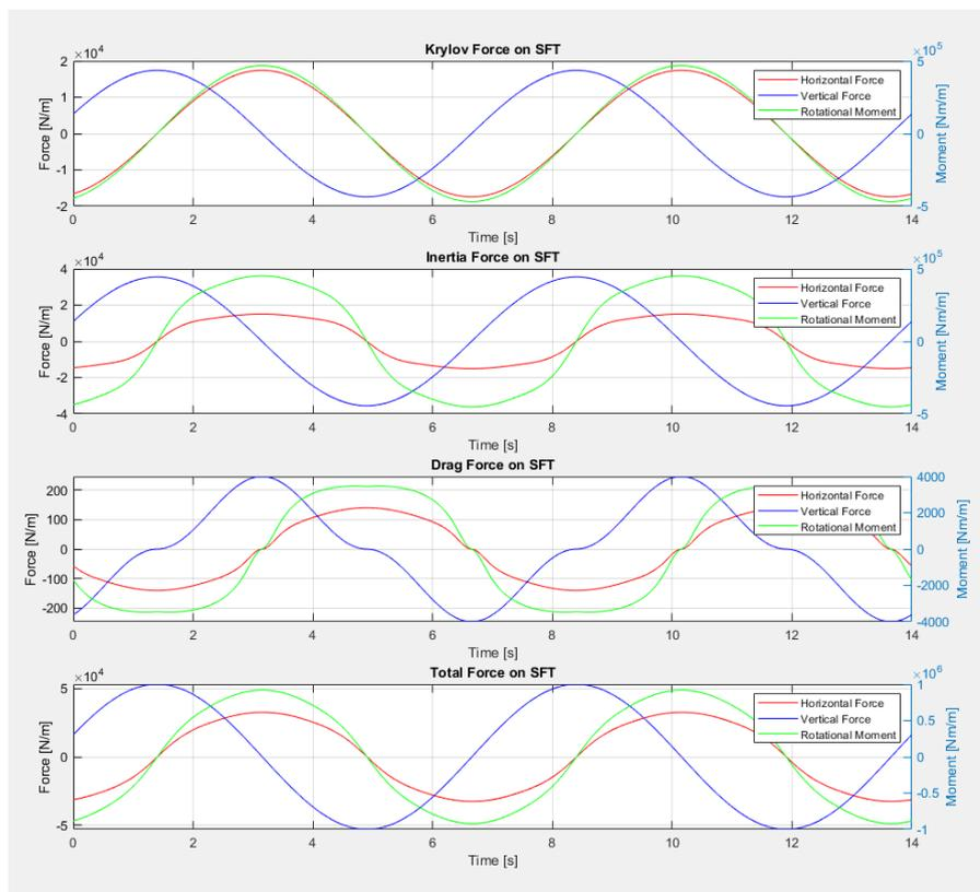
Figure 4.21: The wave loads on a representative rectangle at 20m depth according to Hemel [18]
