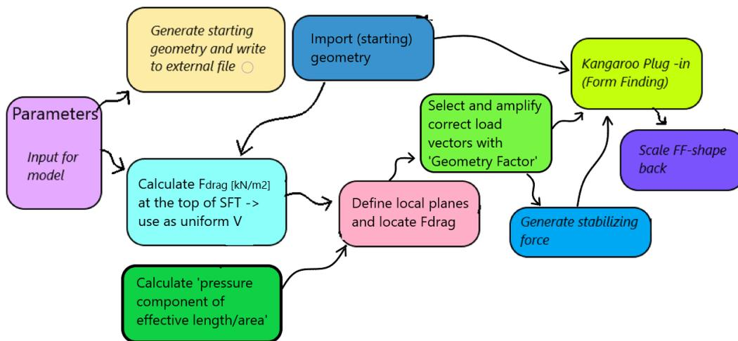
Figure B.7: A schematic overview of the hydrodynamic model for currents in Grasshopper
