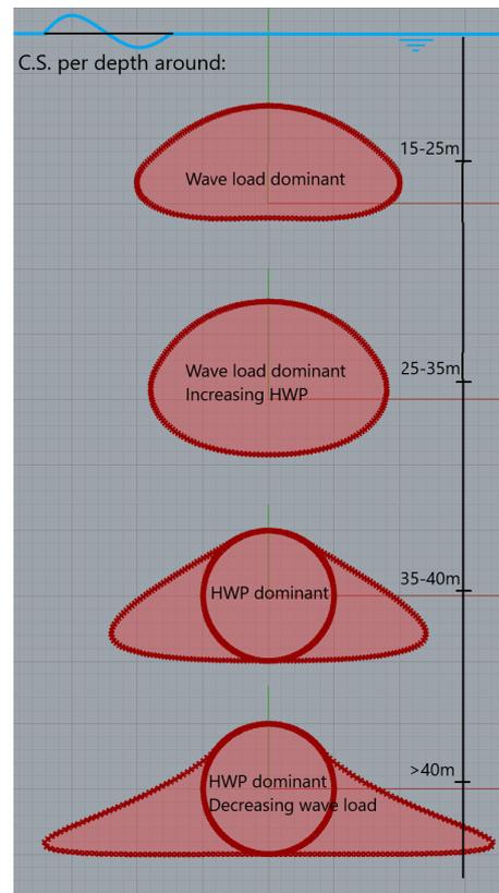
Figure 7.1: cross-section depending on depth
