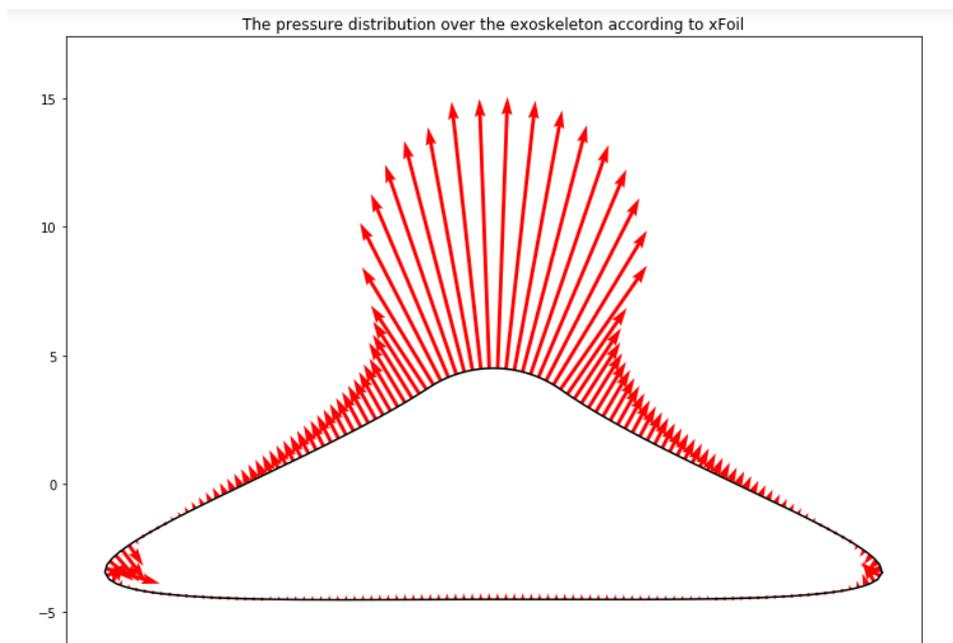
Figure 5.6: xFoil output for pressure distribution
