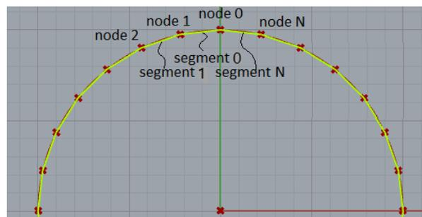
Figure 3.1: The definition of nodes and segments
