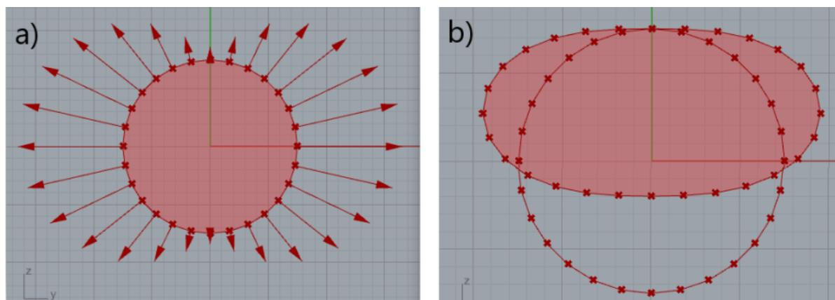
Figure 4.3: a) The load vectors due to currents on the SFT - b) the form-found shape due to this load
