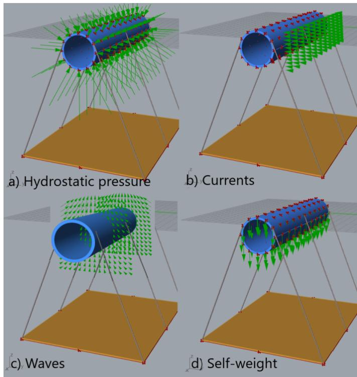
Figure 2.19: The main loads acting on the SFT
