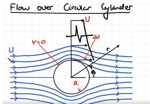
Figure E.1: The analytical flow velocity around a cylinder [16]
