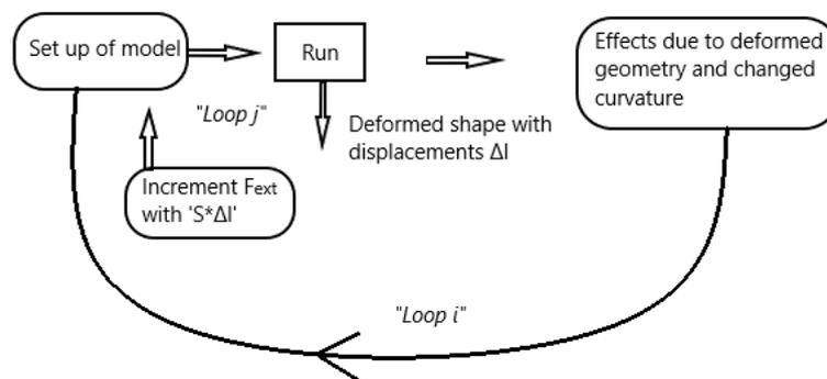
Figure A.5: The double looping process
