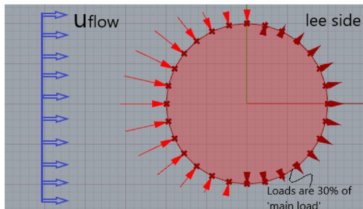
Figure C.1: The load profile for currents
