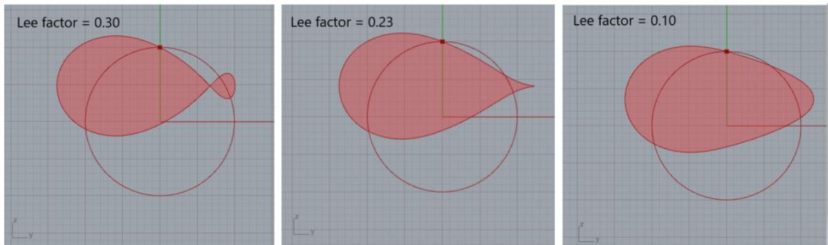
Figure C.2: The FF-shapes for different lee factors
