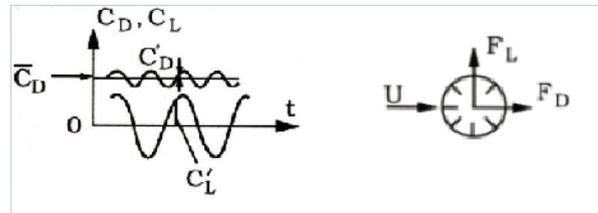
Figure 2.15: The drag and lift coefficients over time [38].
