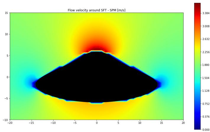
Figure 6.8: The velocity profile for the composite cross-section
