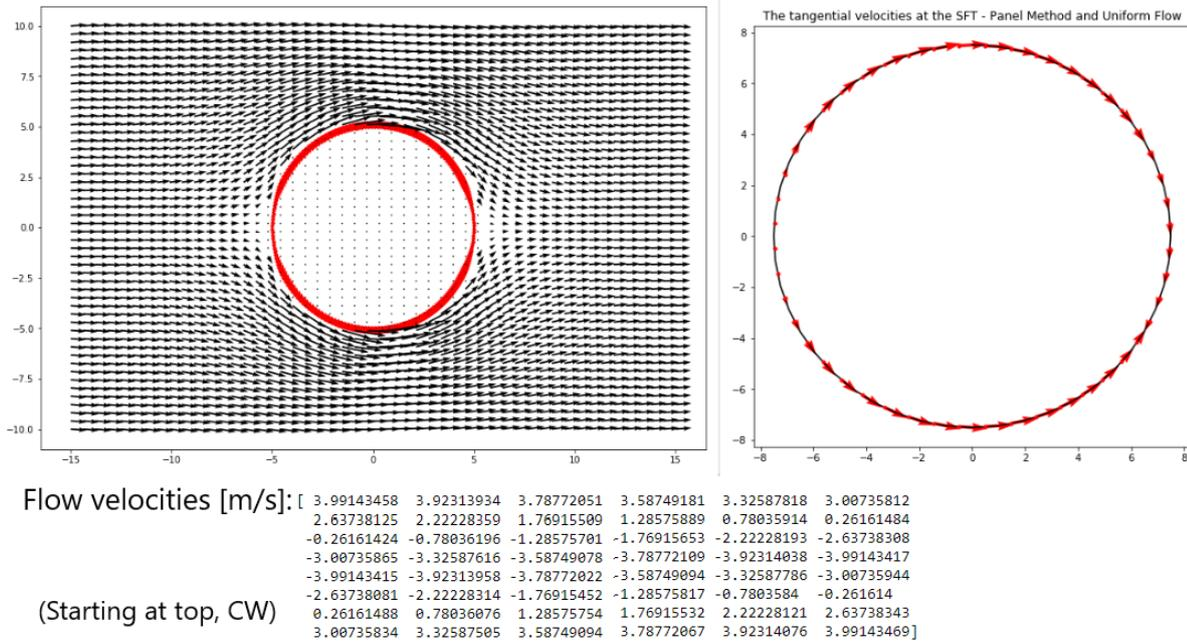
Figure E.5: The flow profile along a cylinder for  $V_{\infty} = 2 \text{ m/s}$
