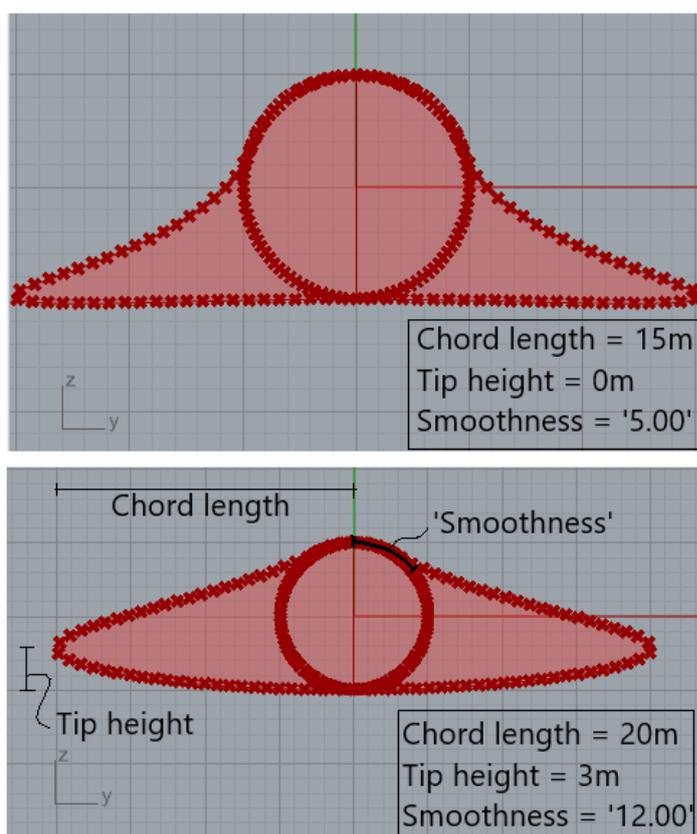
Figure 5.1: The definition of the parameters of the exoskeleton
