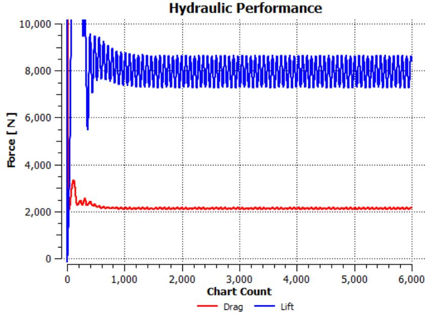
Figure 4.10:  $F_{Lift}$  and  $F_{Drag}$  from the CFD-simulation [43]
