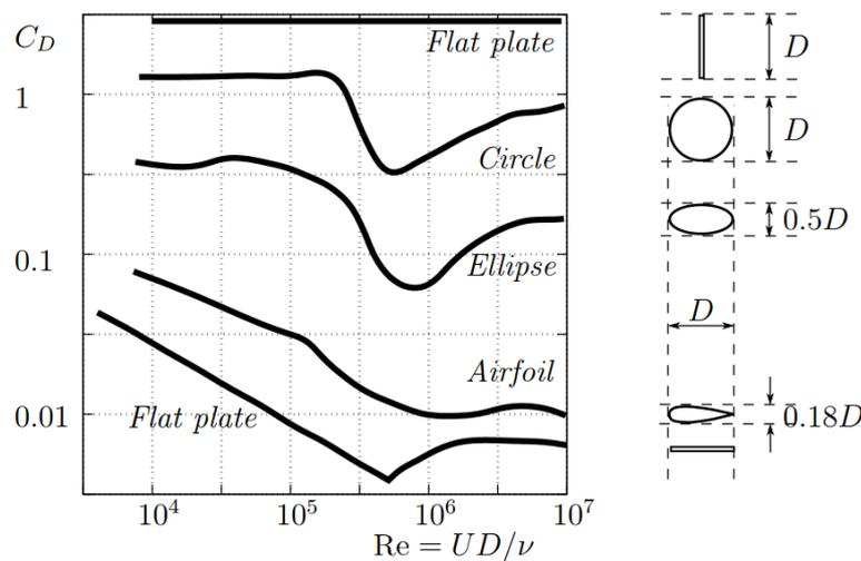
Figure 2.16: Experimental results for  $C_D$  for different cross-sections.
