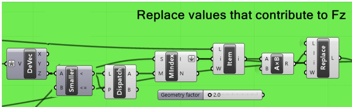
Figure 4.4: The amplification of the load vectors to move the deflection point in Grasshopper
