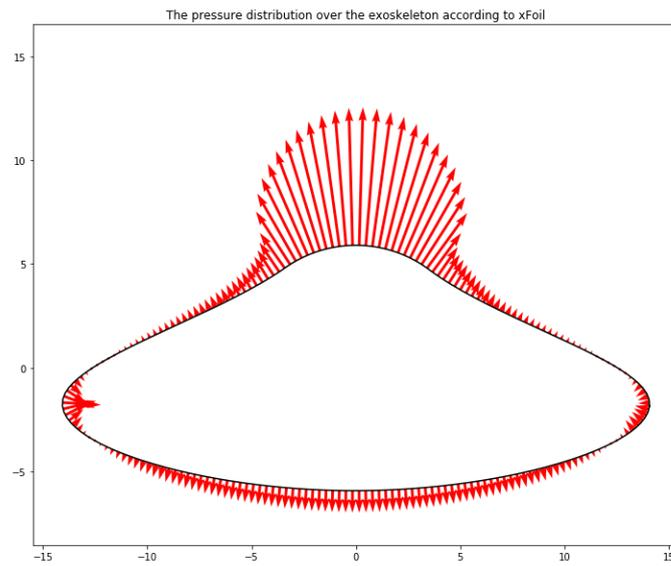
Figure 6.9: The pressure profile for the composite cross-section
