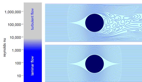
Figure 2.11: The laminar and turbulent flow [7]
