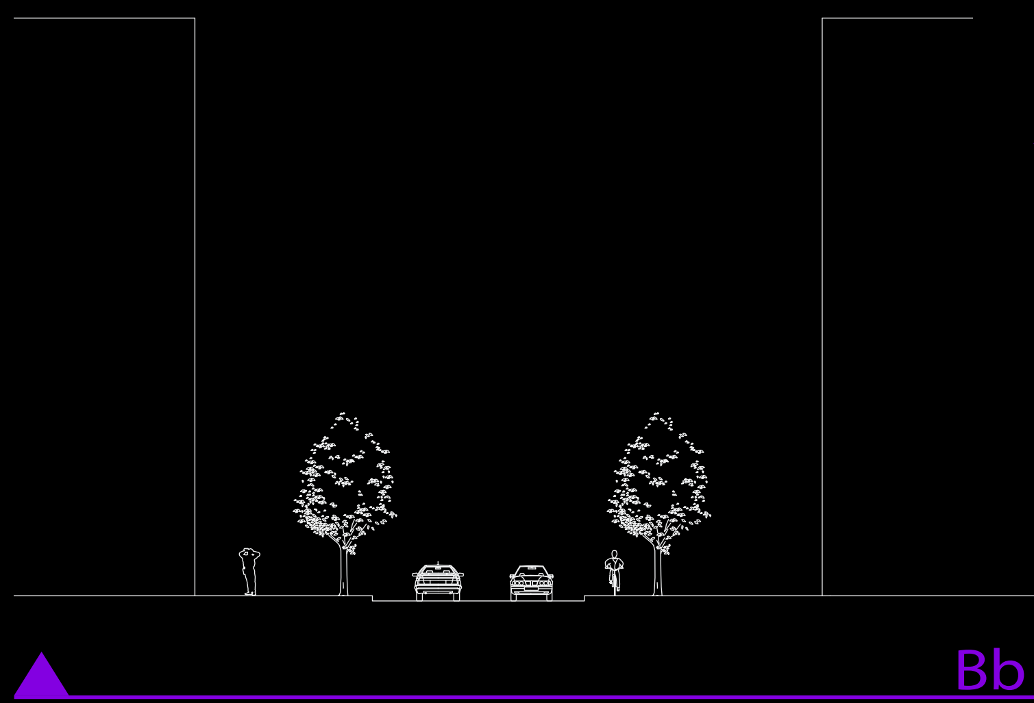
cross section secondary street 0 10m
