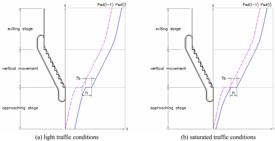
**Figure 3.3** At light traffic conditions (a), flows on escalators depend on arrival processes of pedestrians, while at saturated situations (b) boarding time becomes a determinant to flows or capacities of escalators.
