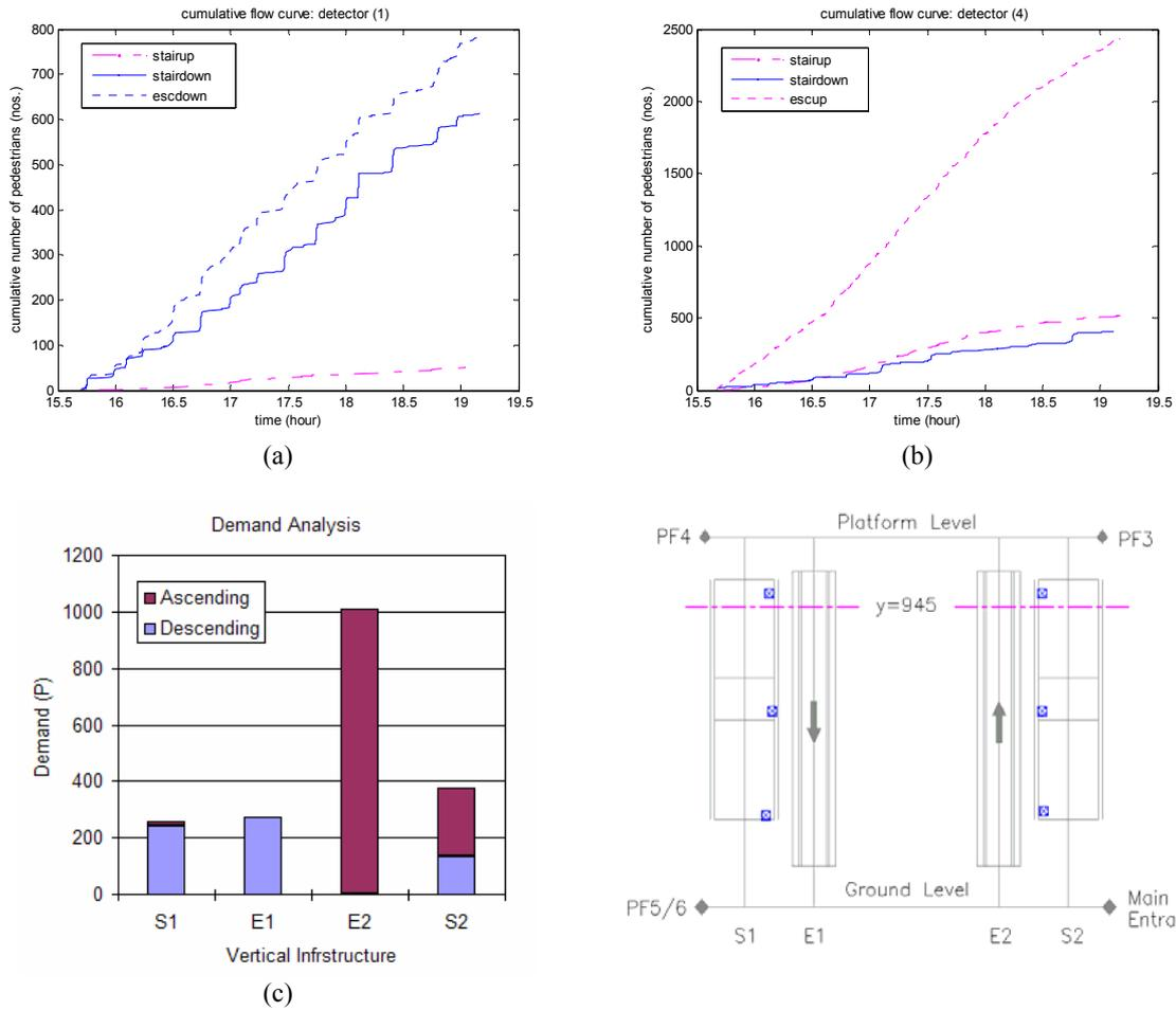
**Figure 5.3** Traffic demands during the observation period from 15:40 to 17:10 (a) cumulative flow curves of infrastructure S1 and E1 (b) cumulative flow curves of infrastructure S2 and E2 (c) traffic demands based on infrastructure types and the direction of movement. Flows are counted at the location of about three steps down the platform level ( $y=945$ ).
