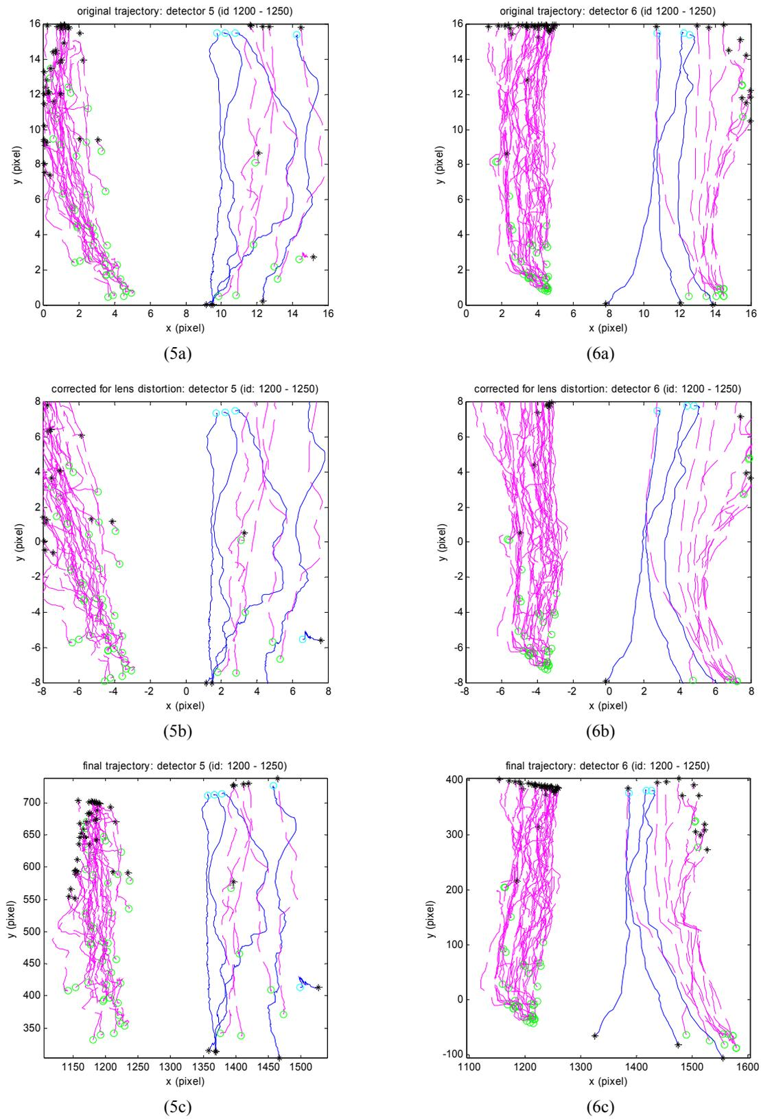
**Figure 6.10** Trajectory plots for Detector-5 and Detetor-6. (5a) & (6a): original plots; (5b) & (6b): plots after correcting for lens distortion; (5c) & (6c): final trajectory plots.
