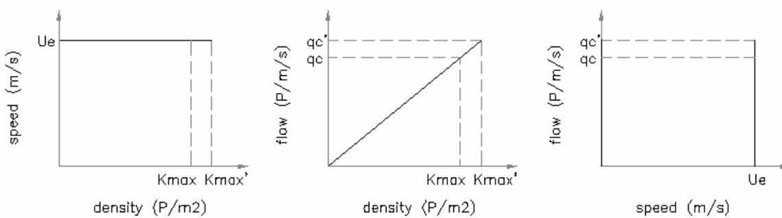
**Figure 3.4** Fundamental diagrams of escalator flows only consisting of standing passengers:  $k_{max}$  and  $k_{max}'$  are the maximum density in the up and down direction;  $U_e$  equals to the operating speed of escalators;  $q_c$  and  $q_c'$  are capacities in the up and down direction.
