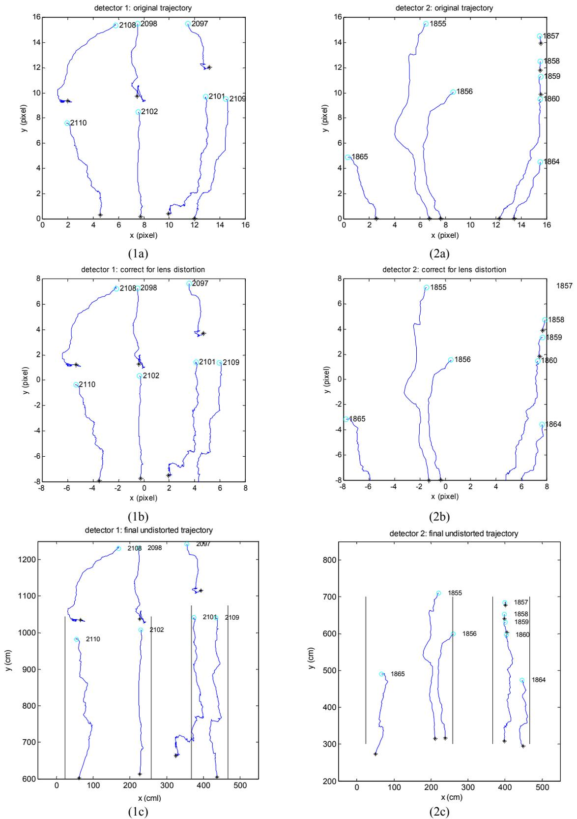
**Figure 6.7** Plots of trajectories; (1a) & (2a): original plots; (1b) & (2b): plots after correcting for lens distortion; (1c) & (2c): plots after correcting for lens distortion and perspective distortion. Besides, the first and final detecting points of a specific target are indicated by the symbol “o” and “\*” respectively.
