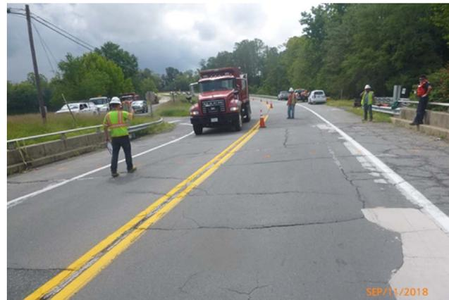
**Fig. 2.** Proof load test on bridge with cracks in overlay along joints of the box beams. (Image by Y. Edward Zhou.)
