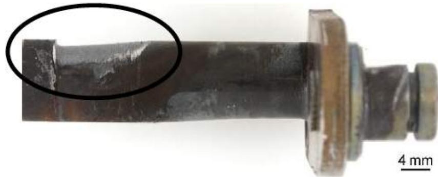
Figure 1.4: Wear damage on the surface of a wastegate lever [3]
