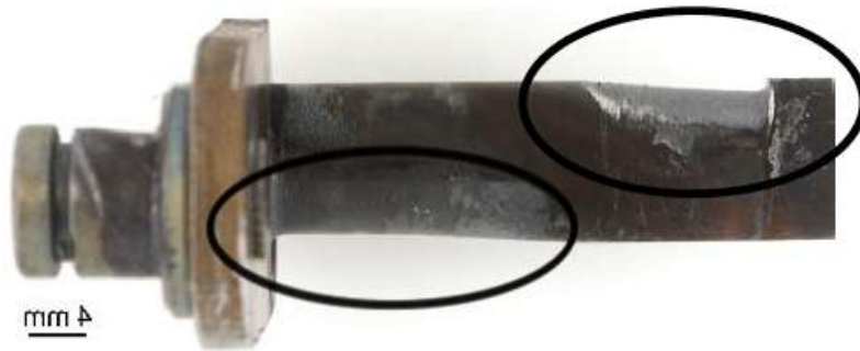
Figure 6.16: Wear damage on the surface of a wastegate lever [3]
