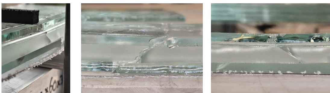
Figure 36: Images showing crack distribution 3-point-bending (own images)
