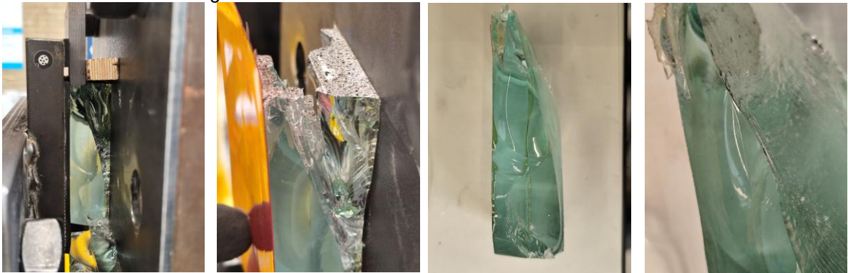
Figure 33: Shear test samples S1-W50: Images showing the crack distribution
