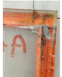
Figure 53: Before and after heating the wire. The thermal shock caused a crack between the glass spacer and the top glass pane (own image)
