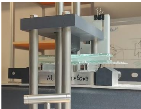
Figure 34: Setup 3-point-bending test (own images)
