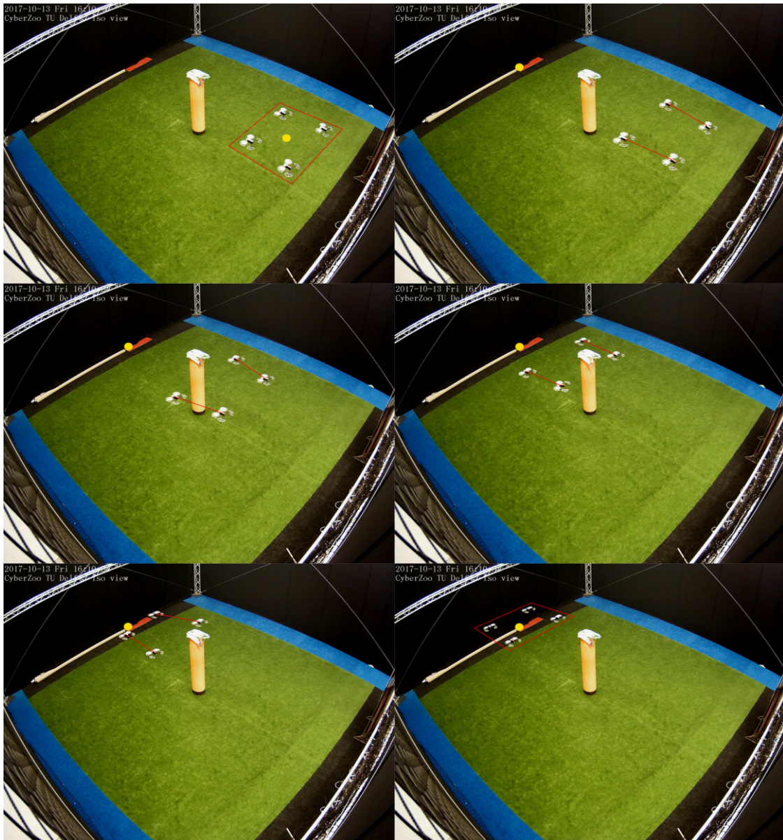
Figure 6-7: Isometric view. From left to right, top to bottom. Snapshots of the UAV team avoiding static obstacle by splitting and afterwards merging. Reference in yellow. Formation shape as red lines.
