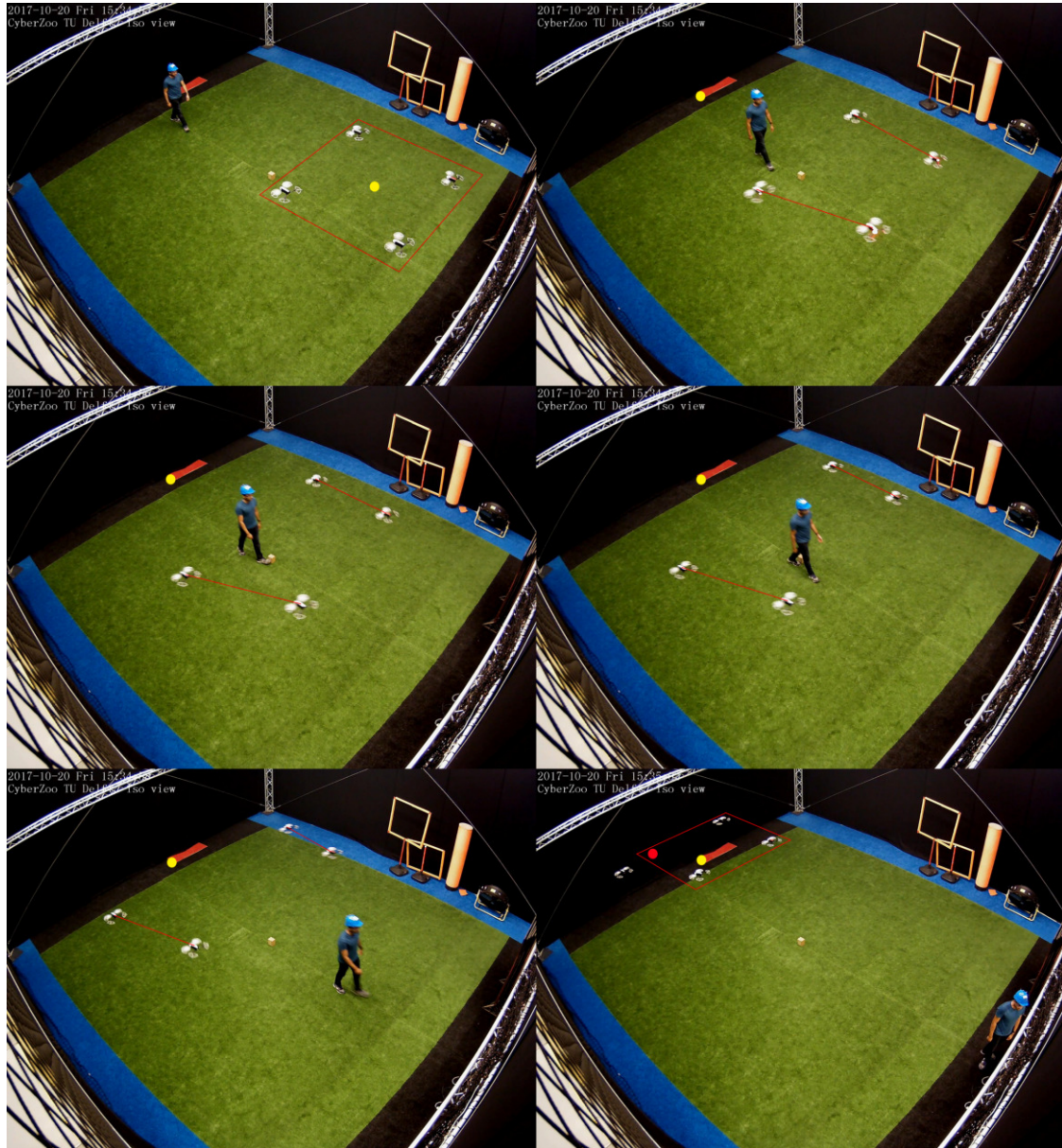
Figure 6-9: Isometric view. From left to right, top to bottom. Snapshots of the UAV team avoiding a moving human by splitting and afterwards merging. Reference in yellow. Formation shape as red lines. Target position for the drone out of position as a red dot (bottom right snapshot).
