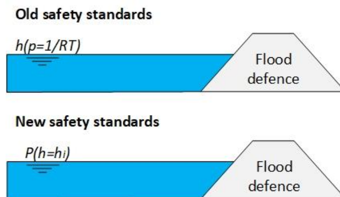
Figure 5: The old safety standards define a return period (RT) of the hydraulic loads. The new safety standards relate to the uncertainty in the occurrence of a certain load ( h_i ).
