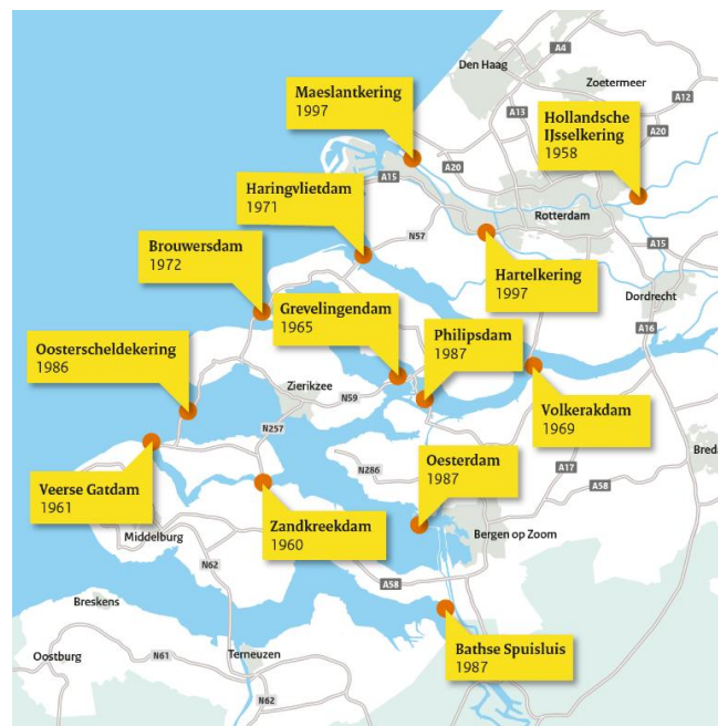
Figure 24: Flood defences in the southwestern part of the Netherlands that are part of the Deltawerken (Rijkswaterstaat, n.d.a).
