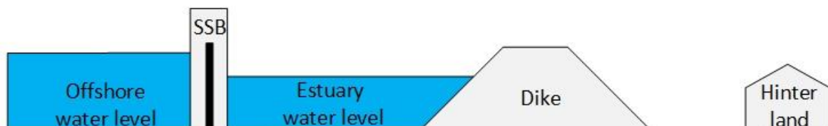
Figure 15: Cross section depicting the elements of the flood protection system.
