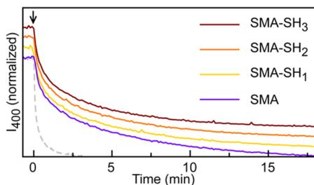
**Figure 2.** Liposome dissolution by SMA-SH<sub>x</sub> and SMA proceeds identically. The intensity of 400 nm light scattered by a solution of 0.05 mg/mL DMPC liposomes at 20 °C diminishes upon addition of up to 0.15 mg/mL SMA or SMA-SH<sub>x</sub> at  $t = 0$  (indicated with an arrow). Each curve is normalized to the initial intensity and offset to facilitate comparison. The dashed gray line shows diminishing of light scattering upon addition of SMA at 25 °C.
