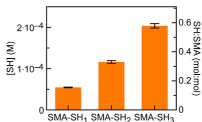
**Figure 1.** Ratio of SMAnh to cysteamine used in the reaction tunes the amount of sulfhydryls in SMA-SH. The concentration of sulfhydryls in SMA-SH<sub>x</sub> solutions of 2.6 mg/mL was determined using the Ellman's assay; error bars show the standard deviation of duplicate measurements. The concentration of polymer was calculated using a molecular weight of 7500 g/mol.
