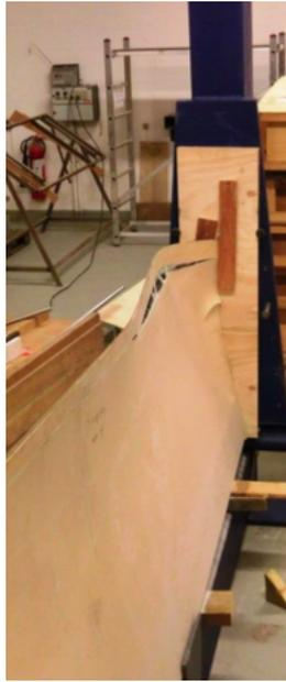
**Figure 3.5:** Figure 2.3b included here for convenience. Buckling and failure of the trailing edge during the first test. [3]
