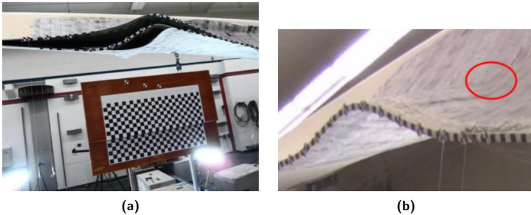
**Figure 2.10:** (a) Ultimate failure from debonding induced by local buckling waves [3]. (b) Trailing edge deformation before attaining the ultimate load. A kink appeared on the top surface (pressure side) [23]
