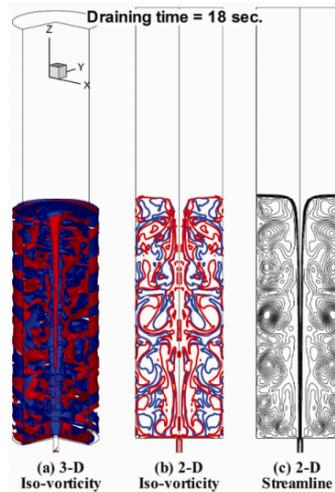
**Figure 1-20:** Vortex streamlines in a fluid draining out of a tank showing Taylor-Like vortices [18].
